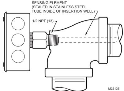
Fig. 3. Method of Mounting C7031D/C7041D Sensor.
