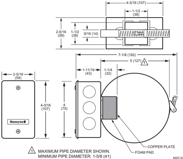
Fig. 7. Strap-on Dimensions in in. (mm).
