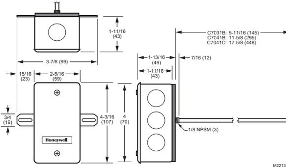
Fig. 1. C7041B,C Dimensions in in. (mm).
