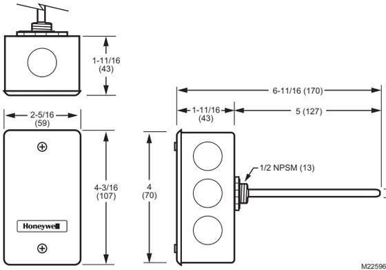
Fig. 4. C7031D, C7041D Dimensions in in. (mm).
