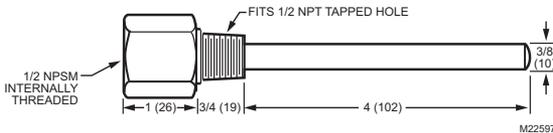
Fig. 5. 50001774-001 Immersion Well Dimensions in in. (mm).
