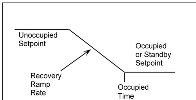
The setpoint ramp will be at the target setpoint 10 minutes prior to the occupied/standby event time. This allows the HVAC equipment an extra 10 minutes to get the space temperature to the target setpoint during recovery.
