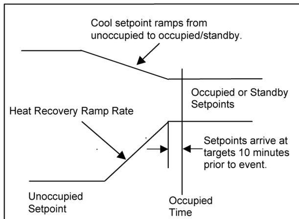
There will be two (2) standard options available for choosing the heating and cooling ramp rates: Single Recovery and Variable Recovery Ramp Rate.
