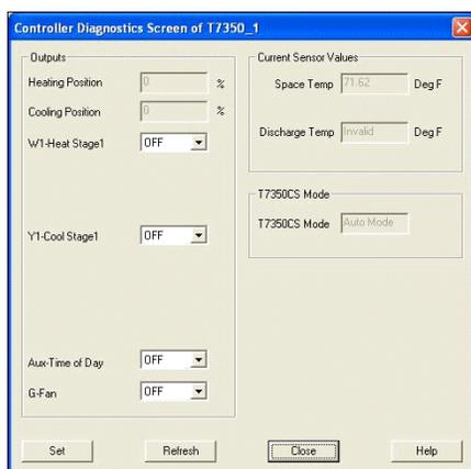
The T7350 diagnostic screen displays the Outputs section where outputs can be commanded, current sensor values to enable the user to watch the effect of the outputs on the various values, and the current mode the T7350 is in.
