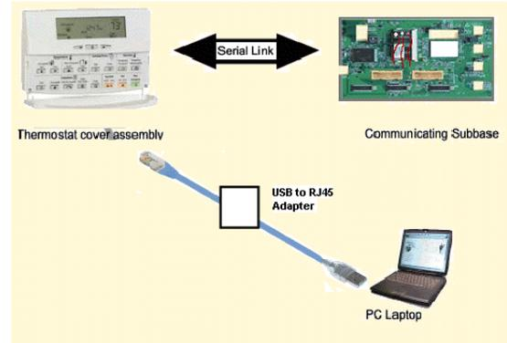
The communicating subbase contains relays, humidity sensor and power supply.
