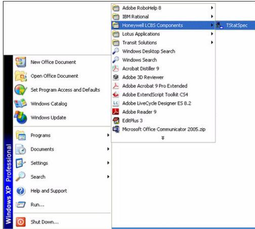
3. Select the folder where TStatSpec™ is installed. Click on TStatSpec™ Folder.
