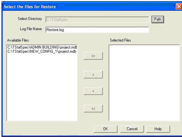
2. Locate the diskette or directory where the backup is stored or the older versions of TStatSpec™ configuration files are located.
