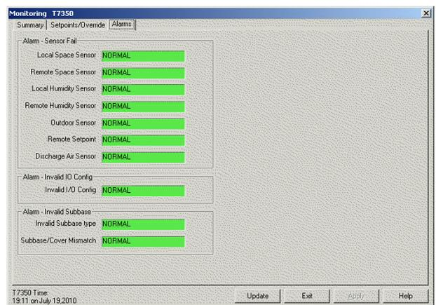
The Alarms screen will display the status of all system alarms and associated errors in the T7350 controller.
