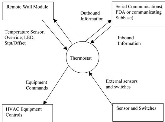
The thermostat has serial communications to allow communications with an installer configuration tool and a future communicating subbase. The thermostat is configured using Installer Setup through the thermostat keys for basic setup functions. More advanced features are available
