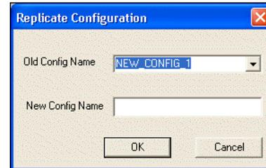
3. From the drop-down list, select the configuration name from which the new configuration database will be replicated.
