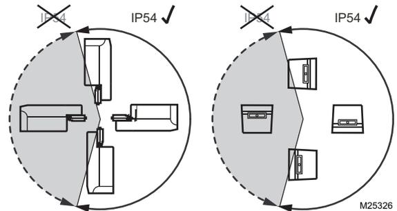
Fig. 8. Mounting for IP54.
