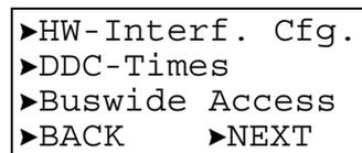
Using the arrow keys, move the cursor to the 'DDC-Times' field. Confirm with ENTER.
