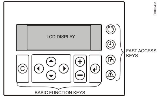
The 'Plant' procedure is used to choose the time program where changes should be made to in the 'Time program' procedure and to make temporary changes to the daily time program. The first screen of the 'Plant' procedure is the start screen. It is the default screen and is always visible when no other screen has been selected. This start screen will also be displayed if no key has been pressed for a long time.
