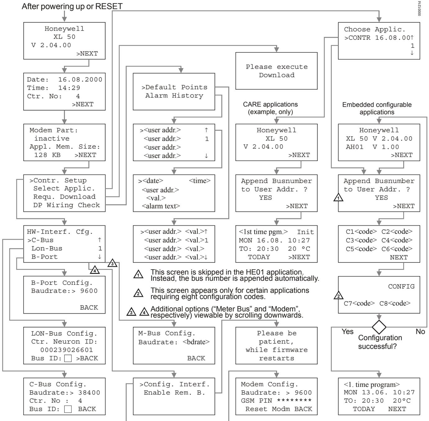
After powering up the controller or after a RESET, the initial screen of the start-up sequence appears. A RESET can be achieved by pressing the 'DOWN' and '-' keys simultaneously.
