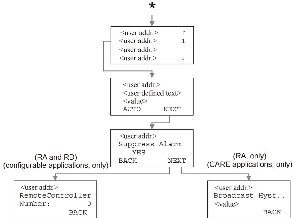
Press the 'Data points / parameters' fast-access key to get access to information on physical, remote and pseudo user addresses, parameters, system data, and the DDC program cycle time.
