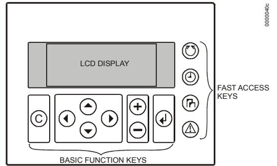
The Excel 50 controller incorporates an operator's terminal featuring a keyboard and a display.
