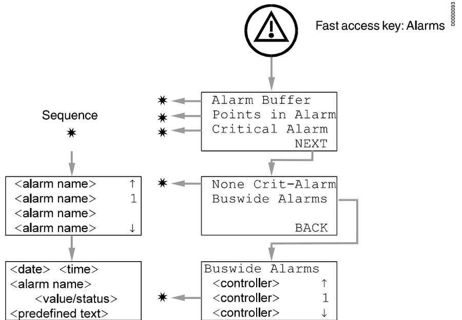
Press the 'Alarms' fast-access key to display alarm information on alarm history, points currently in an alarm condition, critical alarms, non-critical alarms, and buswide alarms.
