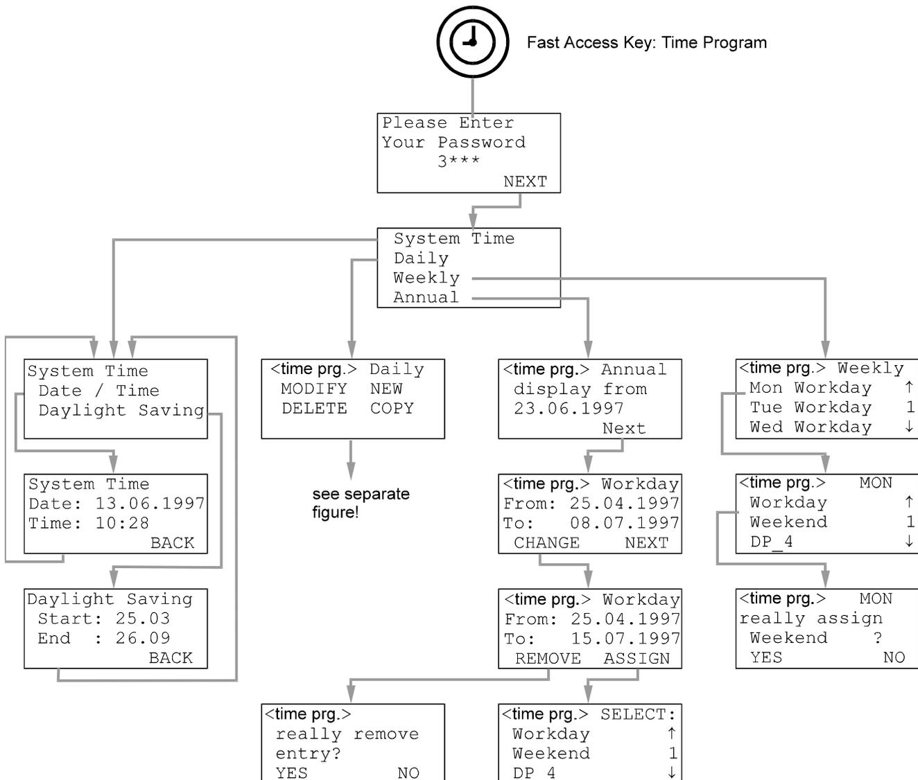
Select the time program by pressing the 'Plant' fast-access key and changing the screens with 'NEXT' until the time program name to be changed appears in the first line of the screen.
