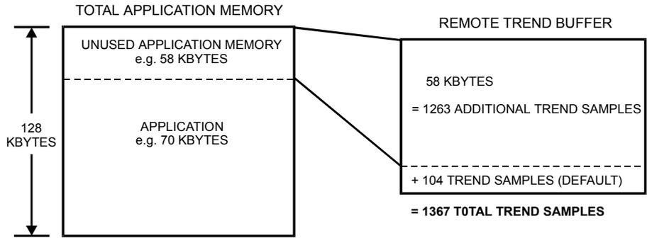
**Figure 1. Adjustable remote trend buffer example.**
