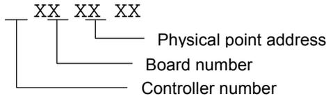
For an explanation of Board Number, see section "Data Point Wiring Check". To enable trend logging for this data point, use the arrow keys to move the cursor to the appropriate field. Confirm with ENTER. Change the value/status using the '+' or '-' keys. Confirm with ENTER.
