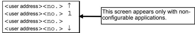
This screen displays the user address and Meter Bus device number assigned to it. To change the Meter Bus device number, use the arrow keys to move the cursor to the appropriate user address and confirm with ENTER. The following screen appears:
