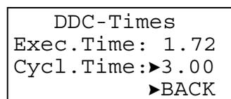
This screen displays the RACL cycle time and execution time in seconds. The cycle time can be changed to optimize the system performance. Changing the cycle time requires a level-3 password. Using the arrow keys, move the cursor to the 'Cycl. time' field. Confirm with ENTER.
