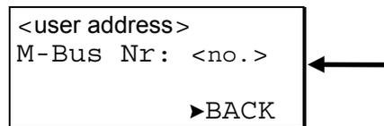
Using the arrow keys, move the cursor to the value field to set the device number of the Meter Bus. Confirm with ENTER.
