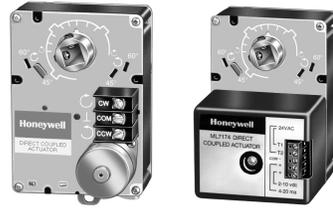
The 35 and 70 lb-in. Non-Spring Return Direct Coupled Actuators (DCA) are control motors that provide floating or proportioning control for valves and dampers. The proportioning motors accept a current or voltage signal from a controller to position the damper or valve at any chosen point between fully open and fully closed.
