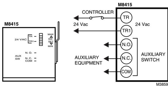
**Fig. 20—M8405 Damper Actuator three-position wiring connections.**
