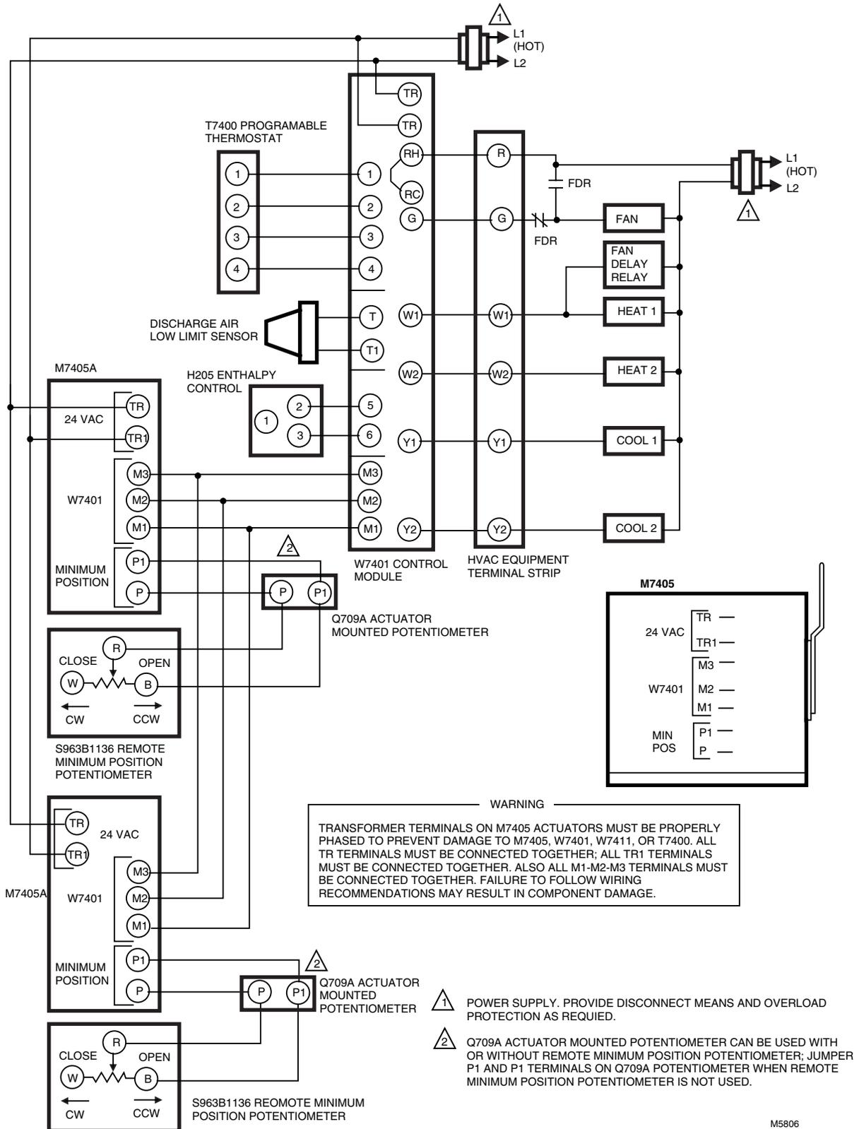
Fig. 5—M7415 Damper Actuator connected in single-stage cooling system with staging relay.
