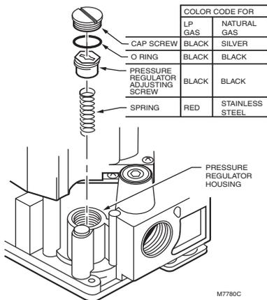
Fig. 4. 393691, 394588 Conversion kit installation in regulator
