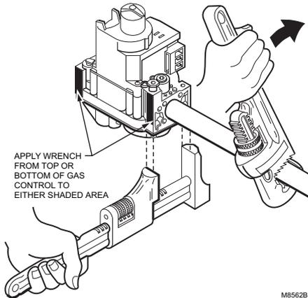
Fig. 6. Proper use of wrench on gas control.
