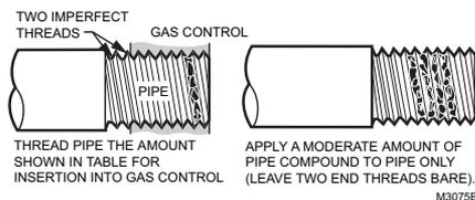
**Fig. 1. Use moderate amount of pipe compound.**
