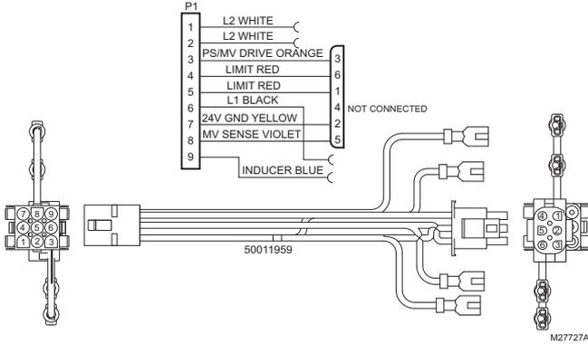
**Fig. 7. ST9101 wire harness adapter 50011959 schematic.**
