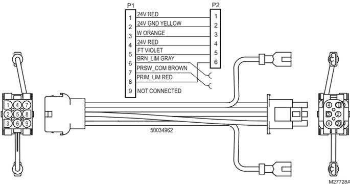
**Fig. 8. ST9141 wire harness adapter 50034962 schematic.**
