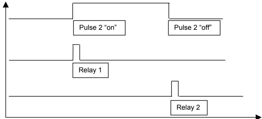
Fig. 3. Pulse 2 flexible data-point switching
