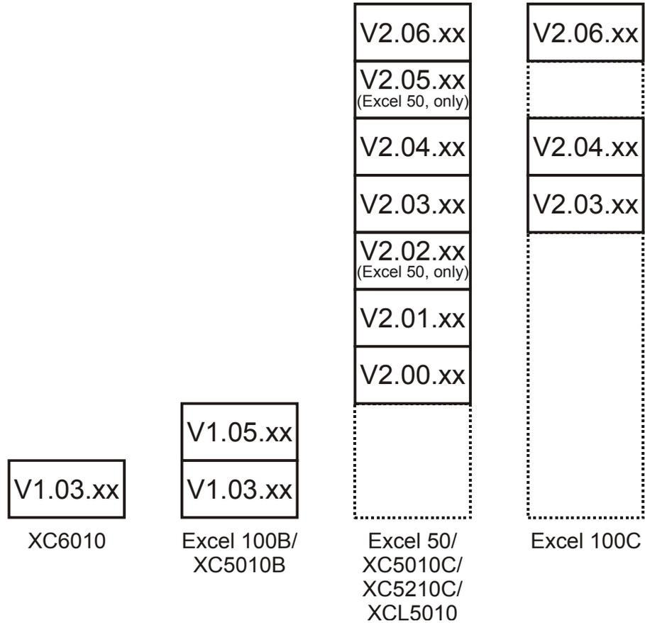
**Fig. 1. Controllers and their supported firmware versions**
