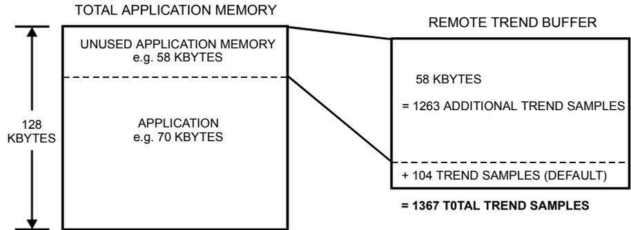
Fig. 25. Adjustable remote trend buffer example
