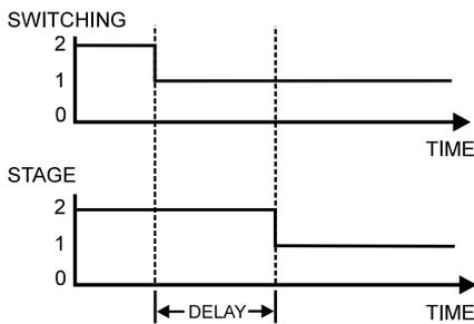
Fig. 9. Delay time switching down
