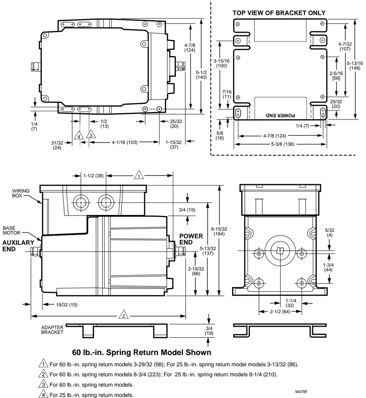
Fig. 1. M4185/M4186/M8175/M8185 mounting dimensions in in. (mm).
