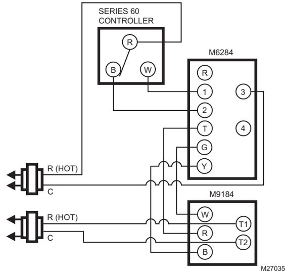
Fig. 10. Series 60 and Series 90 in Slaving Application
