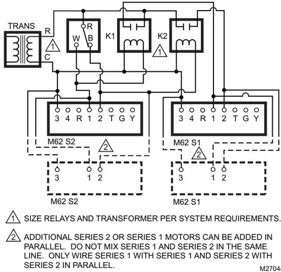
Fig. 9. Series 1 and Series 2 Parallel Application
