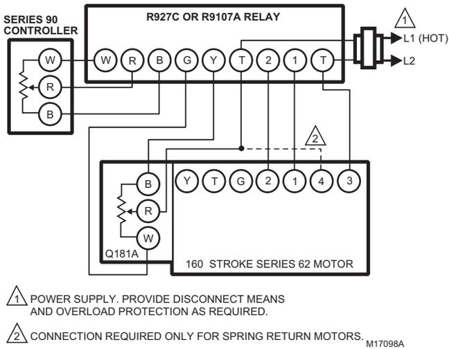
Fig. 8. Connections to R927C or R9107A Relay.
