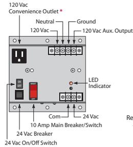
\* Move internal jumper to "HOT" position if you wish outlets to always be hot otherwise outlets will be switched by main breaker.
