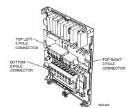
Fig. 3. Re-install terminal blocks
