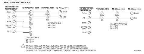
Fig. 7. Wiring examples of three remote wall mounted room sensors for averaging applications
