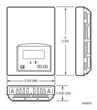
Fig. 10. Thermostat dimensions in inches (mm)
