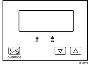
**Fig. 9. Zoning model thermostat buttons and display**
