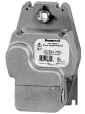
The ML4115, ML8115 Fast-Acting, Two-Position Actuators are spring return direct coupled actuators (DCA) with an integral junction box for on/off damper control. The actuator accepts an on/off signal from a single-pole, single-throw (spst) controller. Models are available with clockwise (cw) or counterclockwise (ccw) spring return and are designed to operate reliably in smoke control systems requiring Underwriter's Laboratories Inc. UL555S ratings up to 350°F.
