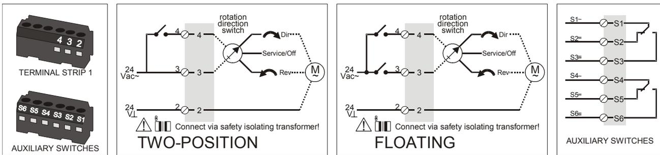
NOTE: Internal auxiliary switches S1 and S4 must be connected to the same power source.
