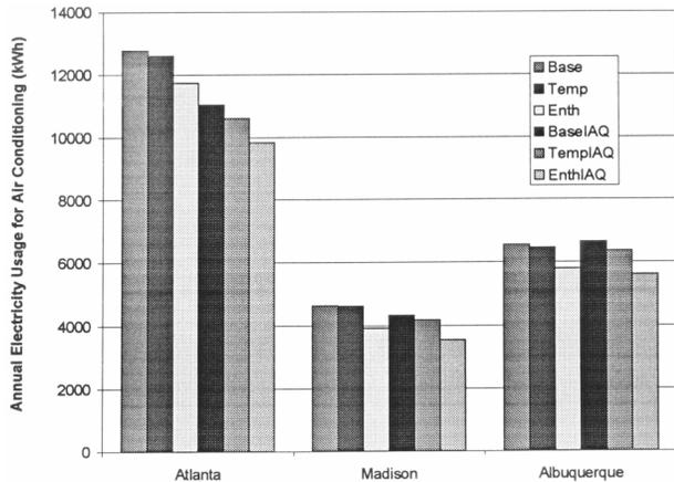
**Figure 3** Annual electrical air conditioning requirements for the office building (not including fan energy).
