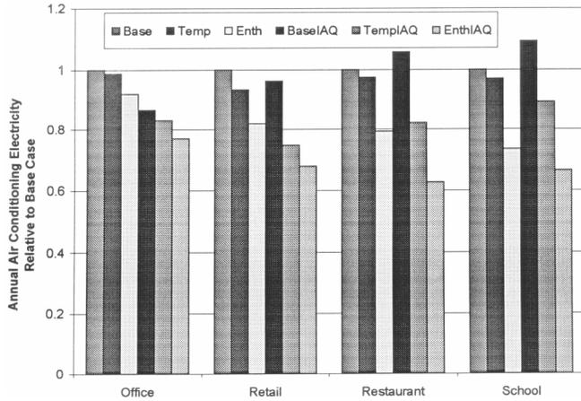
**Figure 6** Annual air conditioning electricity relative to base case for Atlanta.
