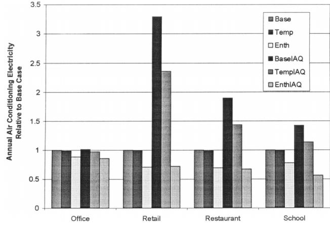
**Figure 7** Annual air conditioning electricity relative to base case for Albuquerque.
