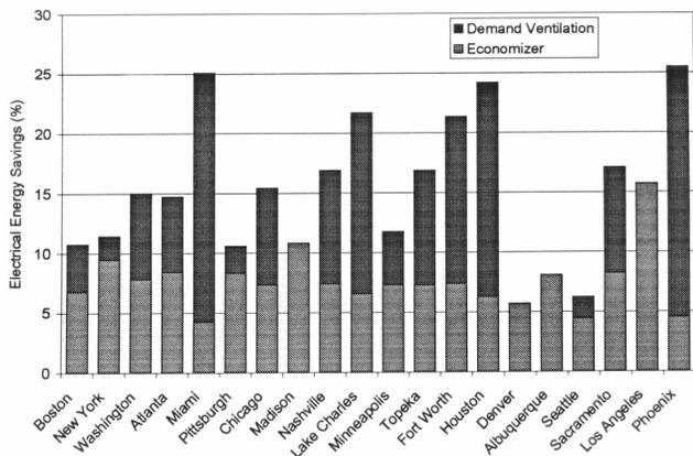
**Figure 11** Incremental energy savings for enthalpy economizer and demand-controlled ventilation (EnthIAQ) for restaurant compared to base case.
