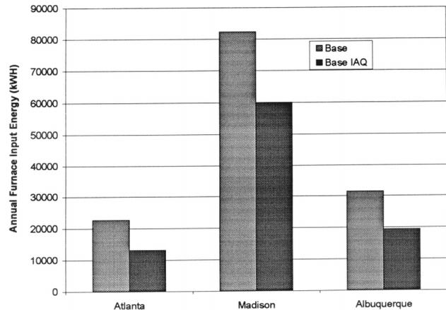
**Figure 4** Annual furnace input requirements for the office building (not including fan energy).
