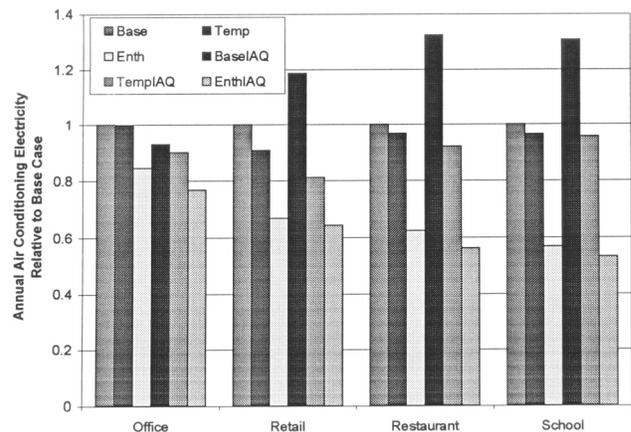
**Figure 5** Annual air conditioning electricity relative to base case for Madison.
