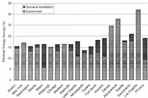
**Figure 12** Incremental energy savings for economizer and demand-controlled ventilation for restaurant with reduced minimum ventilation.
