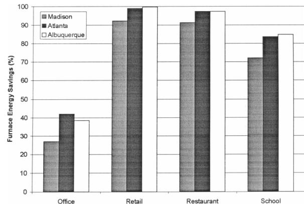
**Figure 8** Annual furnace energy savings for demand-controlled ventilation relative to base case.
