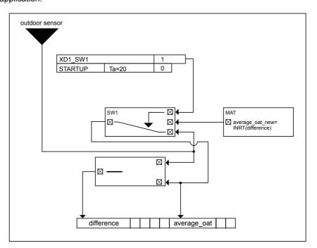
The closed loop control symbol DIF calculates the differential between the momentary outdoor temperature and the old approximate outdoor temperature. The MAT symbol provides a formula to integrate the difference (INT function). The integral function uses TI (reset time) equal to 60 minutes and has a limit value (LIM) of 50C (122F).
