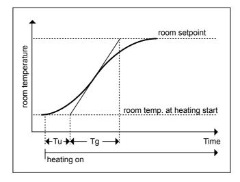
The diagram plots the development of room temperature from heating switch on until it reaches room temperature setpoint. You can draw this type of characteristic curve by recording room temperature (analog input at the Excel controller) and outputting this value to a plotter through an analog output with the characteristic curve 0 through 50 C = 0 through 10V. You need to record separate characteristic curves for preheat after a short cool-down and after a lengthy cool-down.
