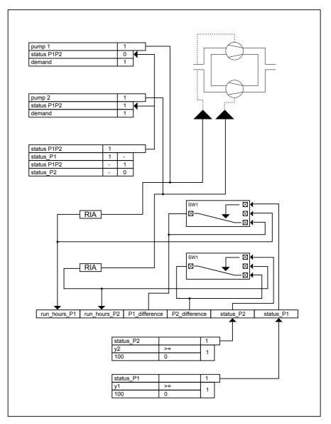
Switchover occurs every 100 hours. The switching tables save the time period for status P1 and status P2. Y1 and Y2 are MAT formulas that work together to operate the switching tables.
