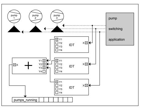
The Y1 output of each IDT connects to an ADD icon that calculates the number of pumps currently running. The ADD output connects to an analog pseudopoint that is available to operator terminals for user display.
