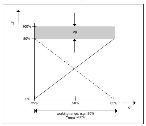
Direct acting signal has a solid line. Reverse-acting signal has a dashed line.
