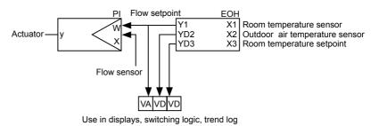
At optimum start, YD2 goes to logic 1 and returns to logic 0 at occupancy start time.
