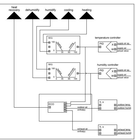
Note that the control loop must reverse the outputs from the temperature and humidity controllers before they connect to the ECO icon. The PID controllers reverse the outputs with the reversed connection of the controlled and reference variable.
