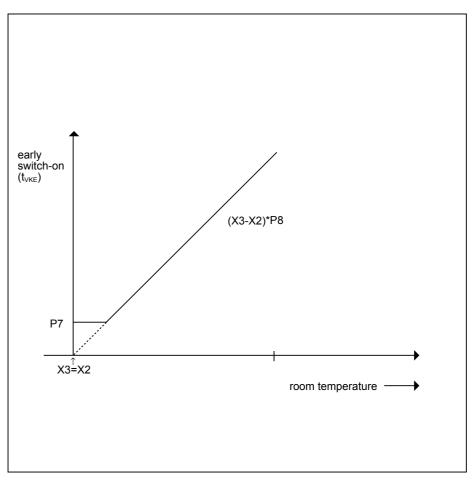
The minimum advancement of start-up is set by Parameter P7 (lowest cooling time for opt. cooling). You must set this parameter to its lowest value so that the calculated start-up point is valid. P7 has a range of 0 to 1080 minutes. The early switch-on time has a maximum limitation of 1080 min (18 hours).
