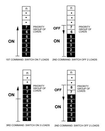
You select the sequential mode of load switching in each priority group by setting Parameters P15 (for Group 1), P16 (for Group 2) and P17 (for Group 3) in XFM 35 to zero. XFM 35 passes these parameters to each XFM 36-1 via the corresponding user addresses ID\_\_\_\_Rotating\_P1, ID\_\_\_Rotating\_P2, and ID\_\_\_\_Rotating\_P3. The user address is not required if only XFM 36-1S is in the priority group.
