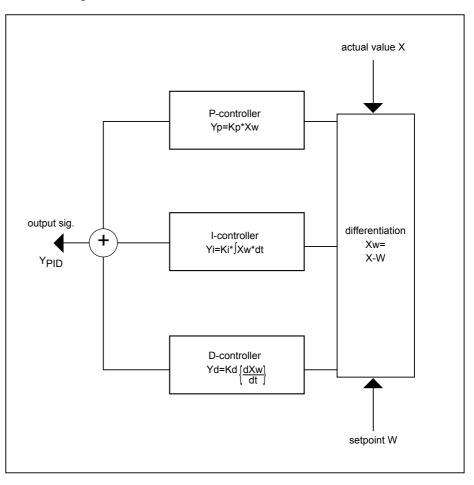
The internal parameters dialog box defines the proportional, integral, and derivative terms as well as minimum and maximum output values that limit the positioning signal (Y). For additional information, see the PID Plus section.
