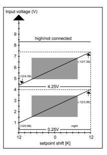
The voltage of the TF26 can move in the gray-shaded areas when the potentiometer knob is turned. Setpoint adjustments of ±degrees Kelvin can be set in the Auto and Day modes of operation.
