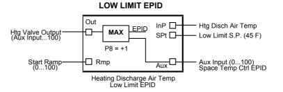
Sequence The space temperature sensor modulates the heating coil control valve to maintain space temperature setpoint. A heating coil discharge air temperature low limit controller prevents the heating coil discharge temperature from falling below 45F.
