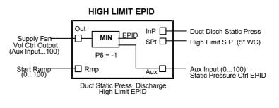
The static pressure sensor located two-thirds down the longest duct run modulates the supply fan air volume to maintain duct static pressure. A duct discharge static pressure high limit controller prevents the supply fan discharge static pressure from rising above the high limit setpoint (5 in. wc).
