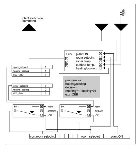
Note that the user address Plant On must be a digital pseudopoint and set by a Time Program to an On or Off value. The ZEB icon decides whether the system is in heating or cooling mode. This example is operated with the corrected setpoint during optimized start-up.
