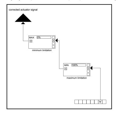
The minimum and maximum values are best input as parameters as shown in the control loop diagram (0 and 100 percent).
