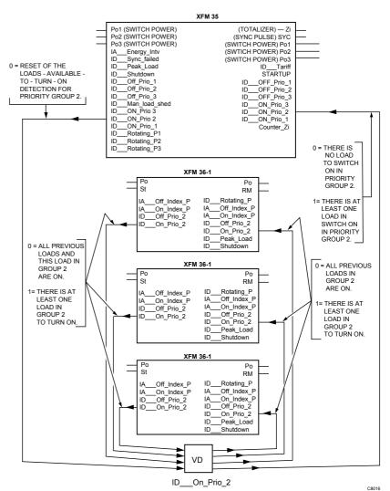
The value of ID\_\_\_On\_Prio\_2 tells XFM 35 if there are any loads that can be restored (turned on) in priority group 2. If not, XFM 35 will not send out a positive kW value on output Po2, but send it to Po1. (If ID\_\_\_On\_Prio\_1 is 1.)
