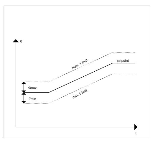
In addition to floating limits, the system should suppress all alarms as long as the supply air fan is off because the supply air sensor cannot measure correct values when the fan is off. The following diagram illustrates both alarm suppression and floating limits.
