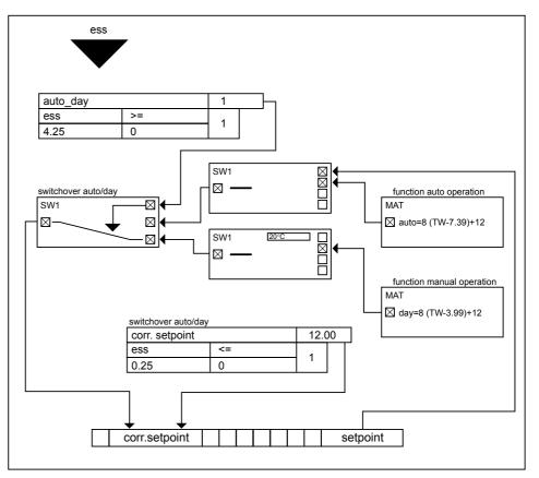
The TF26 temperature selector is represented by the point "ess".
