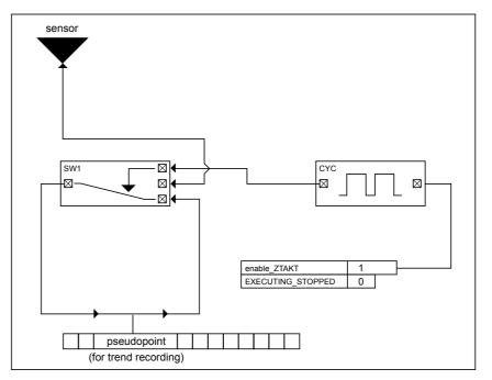
The SWI control icon switches the value of the sensor to the pseudopoint when CYC is in On time. Otherwise, SWI implements a self-hold time for the sensor.
