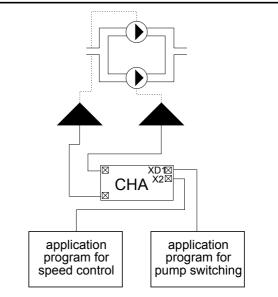
The application programs for speed control and pump switching are control loops with one or more switching tables.
