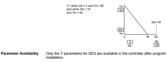
**Negative Values** Use the Ratio (RAMP) function to generate negative values.
