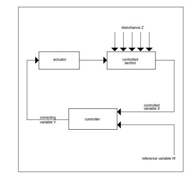
"Disturbance" is the changeable quantity that influences the controller, for example, an outdoor air temperature.
