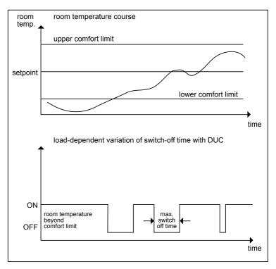
**Off Time Calculation** DUC calculates off time by comparing zone temperatures X1 and X2 with the comfort range (P3). DUC calculates the comfort limits around the setpoint (X4) with the following formulas:
