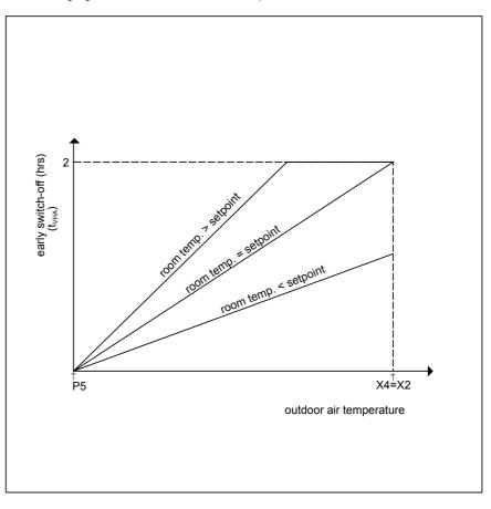
Parameter P6 (optimum stop factor) weights the influence of the control difference on the characteristic curve. If Parameter P6 is zero, EOV calculates early shutdown based on OAT only.
