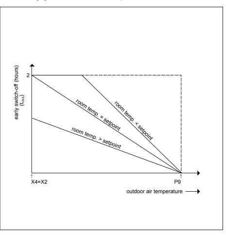
Parameter P10 (optimum stop factor) weights the influence of the control difference on the characteristic curve. If Parameter P10 is zero, EOV calculates early shutdown based on OAT only.
