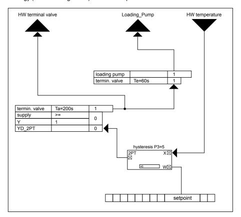
An additional condition is that the common flow temperature of the heat generators is larger than the setpoint plus an increase. This condition is necessary to compensate for piping losses and to prevent the service water storage tank from cooling down because of an excessively low flow temperature, instead of being charged (summer case). This condition is implemented using a switching table that contains a mathematical formula that calculates Y equal to the setpoint plus the increase.
