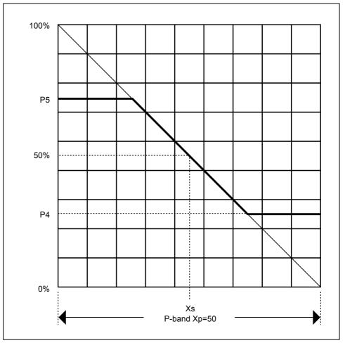
For example, to control a mixing valve that can be open only between 25 and 75 percent (Minimum output and Maximum output), you can set the internal parameters as follows:
