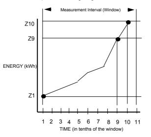
74-5577–10 (US) EN2B-0184 GE51 R0404 (Europe) The algorithm uses the measured energy values (Z<sub>1</sub> Z<sub>10</sub>, and Z<sub>11</sub>) to calculate current power consumption (Parameter P1), possible power consumption (Parameter P4), and finally the power value to be shed or restored by the XFM 36-1/S/R loads (P4 minus P1). (This algorithm does not use display Parameters P2 and P3. Therefore, their values remain zero at run-time.)
