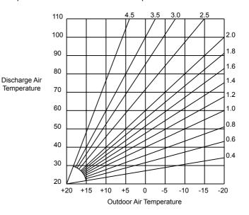
74-5577–10 (US) EN2B-0184 GE51 R0404 (Europe) For radiator heating systems, a heating curve slope 1.6 and curvature 1.33 is the default setting. The higher the curvature value, the more pronounced the curvature. Recommended curvature values :
