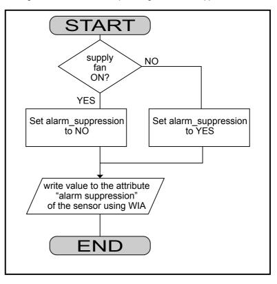
To implement these procedures in CARE, you can use a switching table and a control loop with WIA, ADD, and DIF control icons. The following diagram illustrates the required CARE setup.
