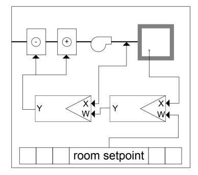
The next diagram illustrates the use of a Cascade controller to perform the same functions. The CAS controller contains two PI controllers in a "cascade" arrangement. The X variable reads the master-controlled variable (room temperature). The XH variable reads the fresh air temperature (auxiliary-controlled variable). The W variable is the room temperature setpoint (reference variable).
