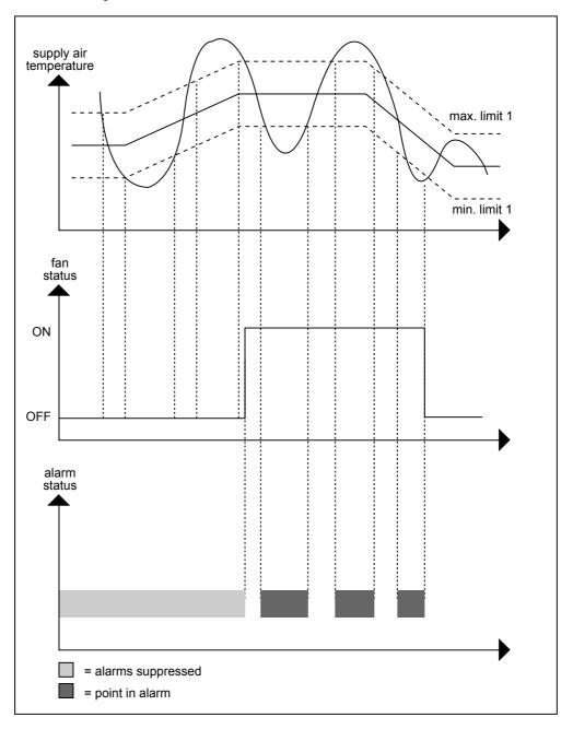
The following flowchart shows the required logic for floating limits.
