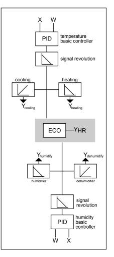
The ECO control icon is composed of six internal modules:
