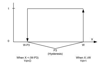
**2PT Example** This example shows how to control a service water storage tank with one sensor. Control action opens the hot water (HW) terminal valve and initiates the release for charging when the actual value of the hot water temperature is less than the setpoint by the amount of the hysteresis. The following diagram illustrates the control strategy (with switching tables) for this example:
