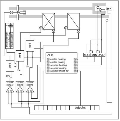
ZEB/Load reset mode is 1 (ZEB) to receive the mixed air damper setpoint.
