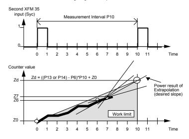
Select the Extrapolation algorithm by setting Parameter P9 to the value 3.
