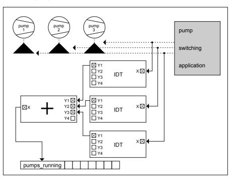
The ADD output now connects to two additional IDT icons to increase the number of connectable analog outputs. One of the additional IDTs outputs to two analog points. The other IDT outputs to two digital pseudopoints. The digital pseudopoints indicate when at least one pump is running.
