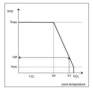
Heating/Cooling System Off Time Calculation
