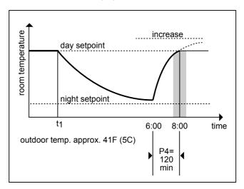
EOH calculates demand flow temperature (output Y1) at the beginning of the preheat phase as a function of outdoor air temperature using a heating curve. If outdoor air temperature changes during the optimization phase, EOH adapts flow setpoint accordingly.
