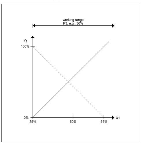
If there is a limitation, the module converts it into a maximum limitation with mixed air damper operation and into a minimum limitation with regenerative transfer operation. Depending on the position of the characteristic curve from Module 3, the positioning signal is direct-acting or reverse-acting. ECO uses the maximum limit for the direct control of mixing, return, and fresh air dampers that operate with one motor.
