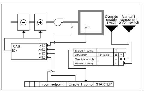
There is an automatic switchover from P control during the start-up phase to PI control during normal operation.
