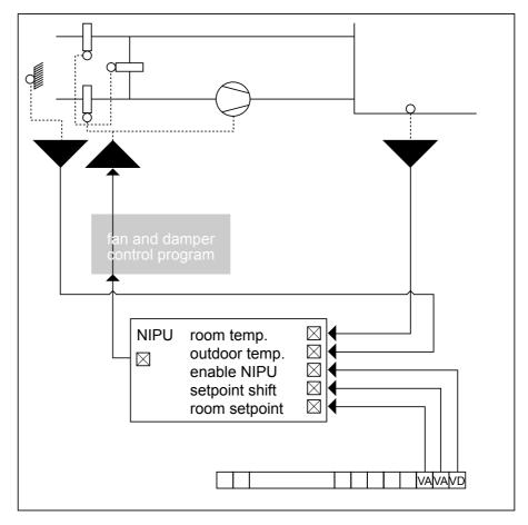
The digital pseudopoint (VD) called Enable NIPU is set by the Time Program in the controller. The Time Program must set it to 1 in the evening (for night cooling on) and to zero in the morning (night cooling off). Because the NIPU has no built-in hysteresis, an independent program for ventilator control (through switch-on delay using switching tables, for example) must perform this function.
