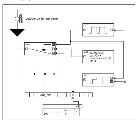
The CYC statement generates a series of impulses with a period duration of 10 minutes (scan time). To do this, the CYC icon must have the following parameter assignments:
