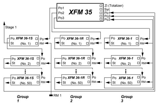
The principle of operation is that XFM 35 implements the desired algorithm and then outputs the actual kW shed/restore values to the XFM 36-1/S/Rs. A positive kW value is a command to restore loads totaling that much kW. A negative kW value is a command to shed loads of that much kW. The kW shed/restore values can appear at output Po1, Po2, or Po3.
