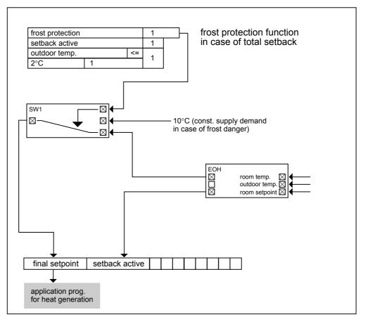
A switching table implements an outdoor air temperature-dependent frost protection function outside of EOH. When outdoor air temperature is less than or equal to 2C (36F), the table sets a constant room temperature setpoint (for example 10C [50F]). The value of the constant is the X2 input parameter of the SWI icon.
