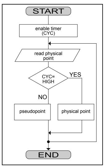
To implement this extended trend function, CYC must be part of a control loop that includes other functions. The following diagram illustrates the complete control loop.
