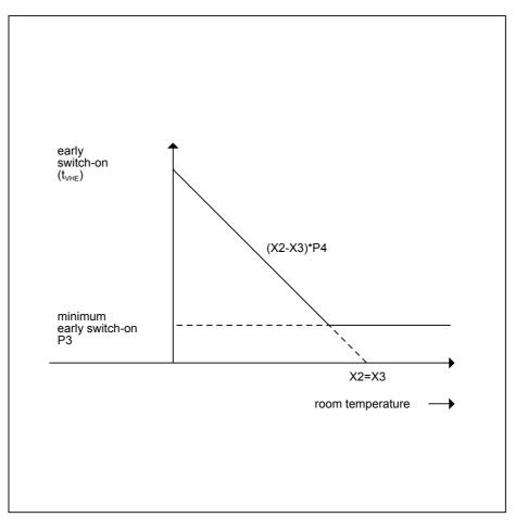
The shortest advancement of start-up is set by Parameter P3 (lowest pre-heat). You must set this parameter to its lowest value so that the calculated start-up point is valid. The parameter's maximum limitation is 1080 min (18 hours).
