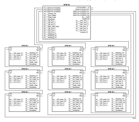
The following diagram shows an example of how datapoint ID\_\_\_On\_Prio\_2 exchanges data between the XFMs.
