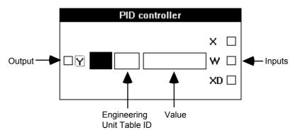
You need to connect the Y, X, and W variables to either physical points, pseudopoints, and/or other control icons. Variables on the left (Y in this case) are always outputs. Variables on the right (X and W in this case) are always inputs. The icon descriptions in the Alphabetic Reference chapter define the types of connection that are valid for each variable.
