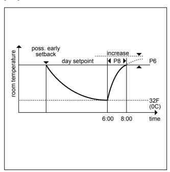
During this preheat phase, EOH transmits a 1 to the output (YD2). You can use this output to determine whether to overwrite the supply temperature setpoint from the normal application program by the flow temperature setpoint (Y1) from EOH.
