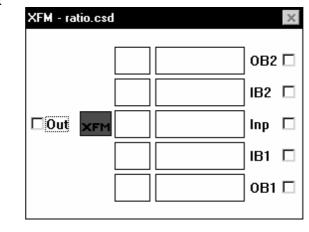
Inputs OB2 = output bound 2 IB2 = input bound 2 Inp = Input IB1 = input bound 1 OB1 = output bound 1
