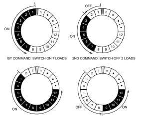
3RD COMMAND: SWITCH ON 5 LOADS 3RD COMMAND: SWITCH OFF 6 LOADS
