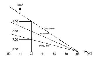
EOH calculates a discharge air setpoint based on the selected outdoor air temperature/discharge air (OAT/DA) schedule (default is 1.6) plus the effect of P8 (parallel shift) and the time program room setpoint it must achieve. During this optimized ON period , the discharge air setpoint varies with the OAT. P5 determines maximum discharge air setpoint.
