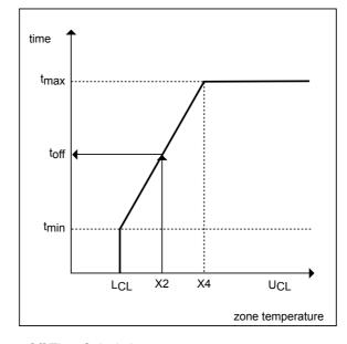
Cooling System Off Time Calculation
