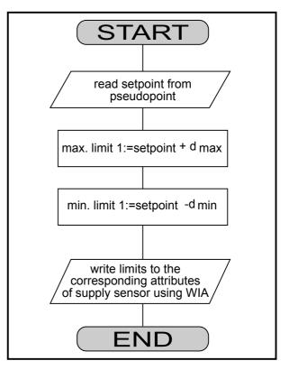
The following flowchart shows the required logic for alarm suppression.
