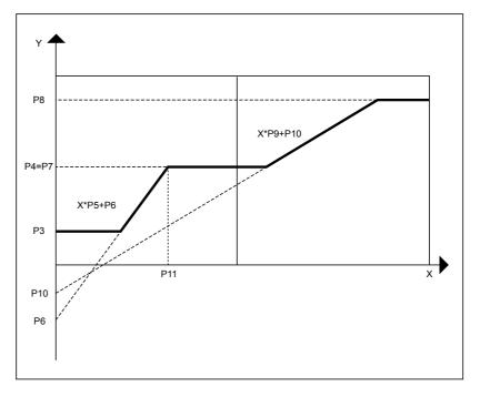
Scale Changes When you change the minimum and maximum X and Y scale values, RAMP adjusts minimum and maximum values for the curves so that they are not outside the overall X and Y ranges.
