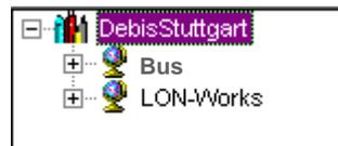
Each bus is sub-divided by default to allow an arrangement of the network components according to the physical conditions in the building.
