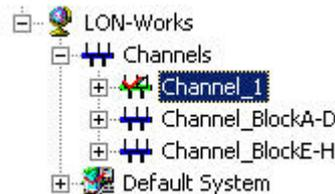
**RESULT:** The selected channel gets green and is now the interface channel via which CARE connects to the LonWorks network when going Onnet.
