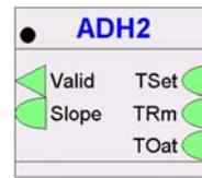
Input ports are red colored, if they are not connected, if they do not get any input. The color green indicates the accurate connection of the port. Pointroles are not a valid connection and must be changed for translation. Thus pointroles are also red.
