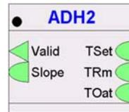
Input ports are red coloured, if they are not connected. The color green indicates the accurate connection of the port.
