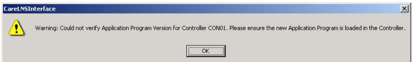
Click the OK button. Connect the controller to the network. Download the correct application into the controller and commission the network.
