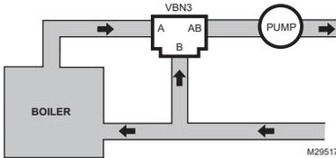
Fig. 4. Reset mixing control for discharge hot water.
