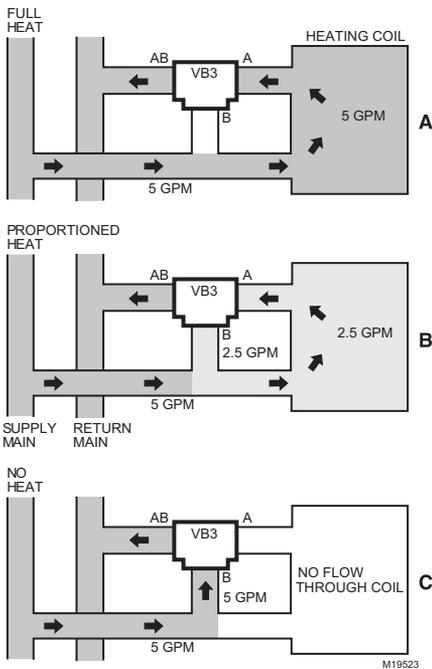
Fig. 5. Three-way mixing valve operation with coil bypass.
