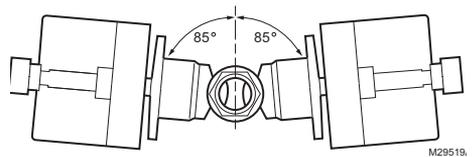
Fig. 2. Acceptable valve angle from vertical.
