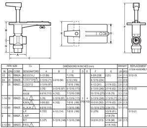
1 INDICATES FULL PORT VALVE: NO FLOW CHARACTERIZING INSERT.
