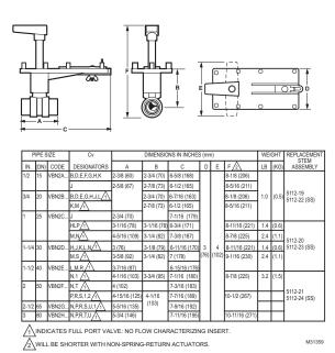
Fig. 8. VB2 dimensions in inches (mm).
