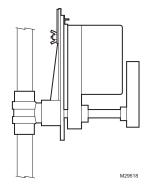
Fig. 1. Vertical valve installation.
