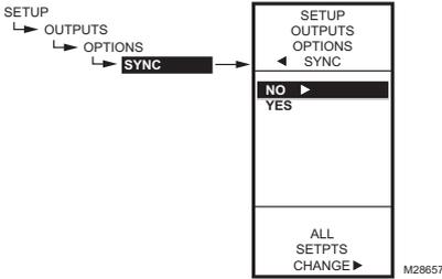
Fig. 62. Installation - Sorties - Options - Sync.
