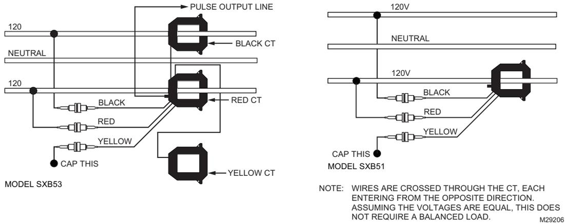
Fig. 9. Typical 240/120 VAC 1Ø, 3-wire installation.
