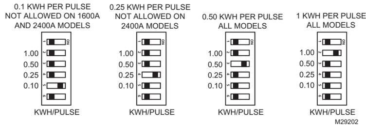
Fig. 5. Setting pulse-rate switches on the meter.
