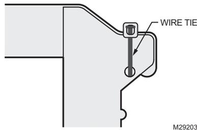
Fig. 6. Use wire ties to secure the I-bar to the CT housing.
