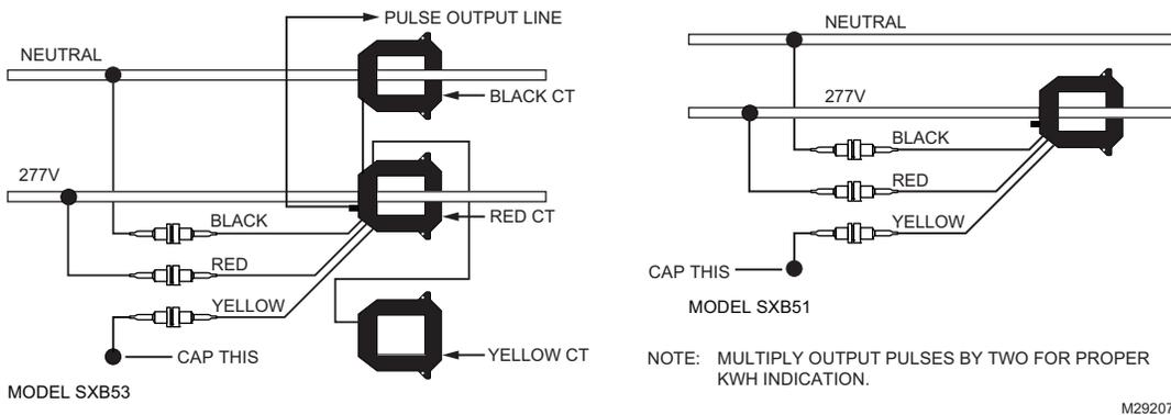
Fig. 10. Typical 277 VAC 1Ø, 2-wire installation.
