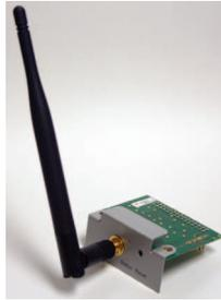
**Fig. 15. Wireless communication card.**
