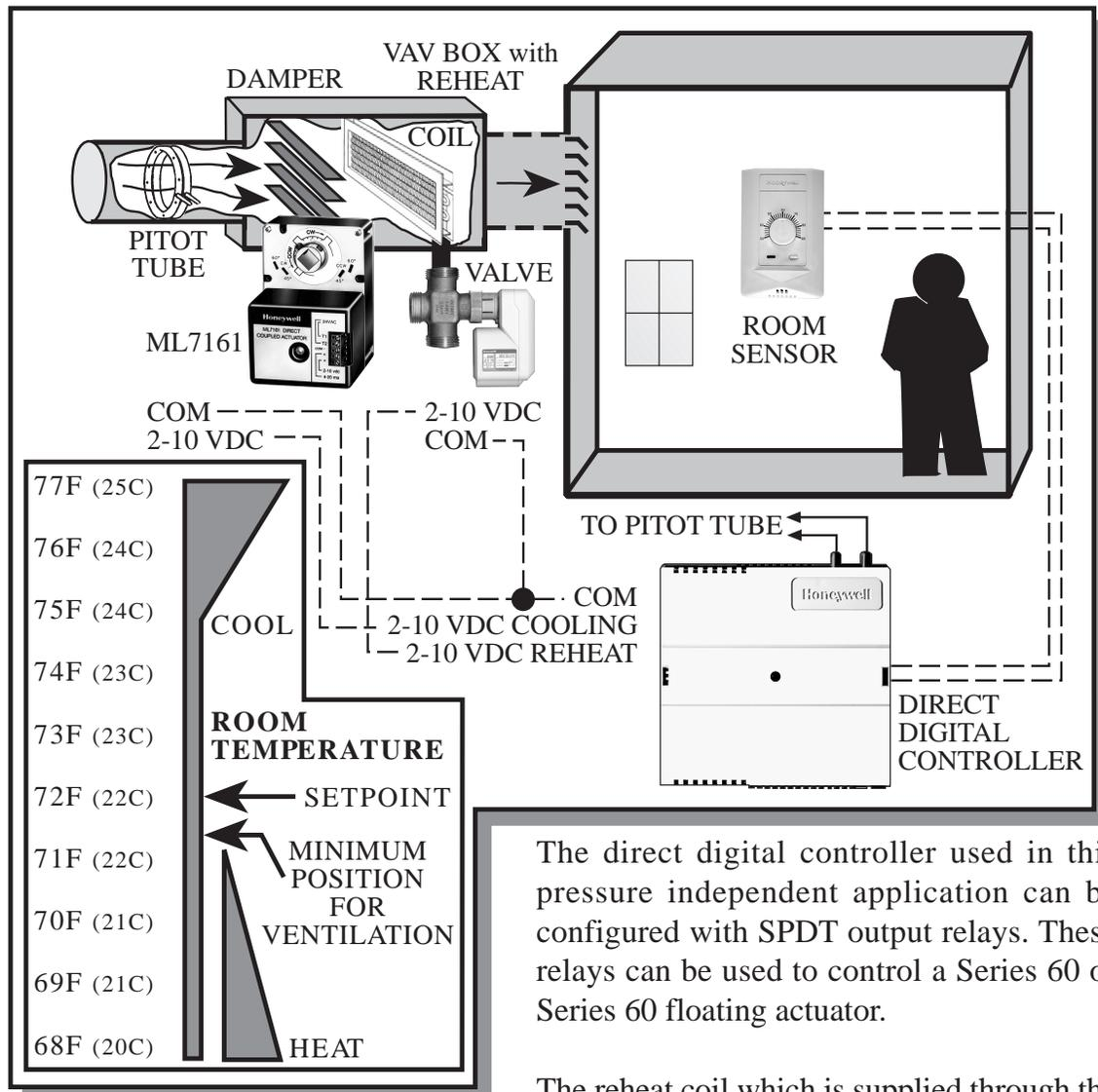
Series 70 devices use 0 to 10 volts dc (Vdc), 2 to 10 Vdc or 4 to 20 milli-amp (mA) control circuits. These control circuit voltages are very prevalent today, making replacement of other company's actuators with Honeywell devices economically feasible. Series 70 is intrinsically modulating with actuator feedback either built into the signal voltage or from a feedback potentiometer. Both actuators in this illustration are supplied with 24 volts AC.
