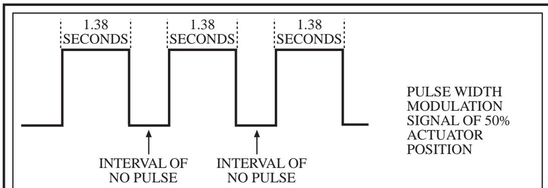
If this control circuit were this type of pulse width modulation:
