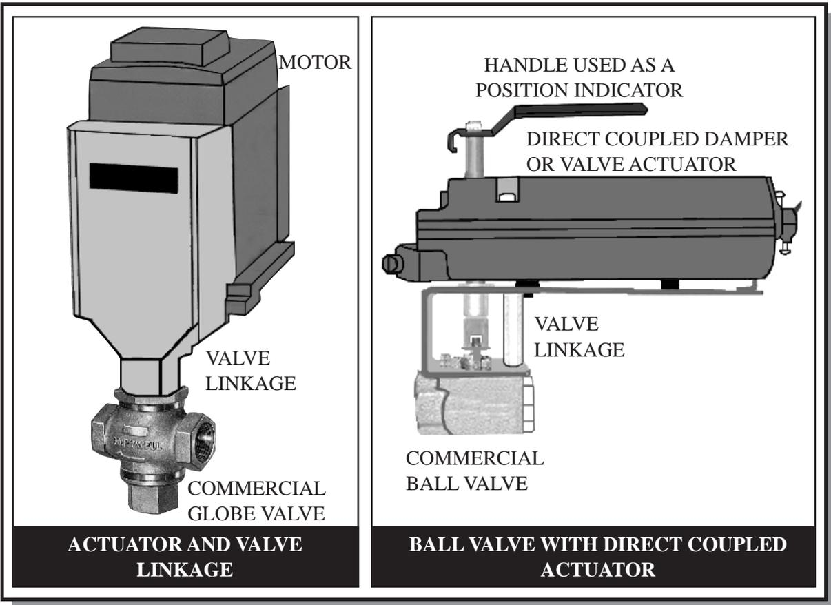
For many years the primary method of controlling a commercial valve with an electric actuator was to use a three piece assembly. It consisted of a valve body, a valve linkage and an electric or electronic actuator.
