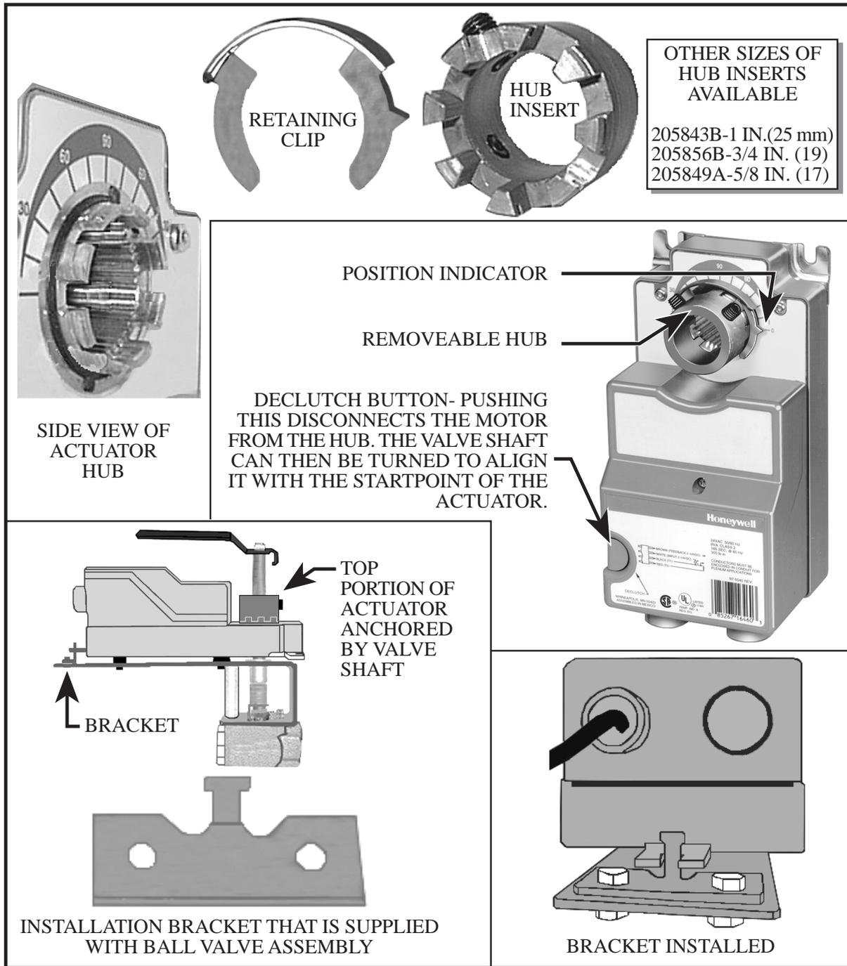
The 300 lb-in (34 N-m) non-spring return actuators are installed on the flat back side only. Direct-reverse adjustments are done on series 70 units with a switch on the side. Hub inserts are available for various shaft sizes but only the 1/2 or 1 inch (13 or
