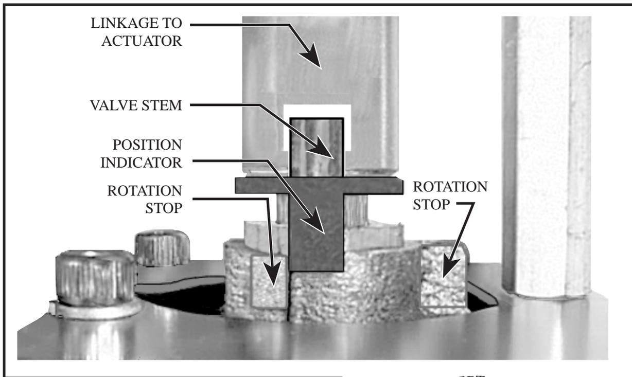
Most ball valve stems are either 1/2 (13 mm) or 1 inch (25 mm). The hub size of the actuator should match the diameter of the stem. This is important since most of the direct coupled actuators are available with various hub sizes. Similar to most globe valves the stem should always be one degree or more above horizontal. Direct contact of moisture or condensation can cause damage to most direct coupled actuators.
