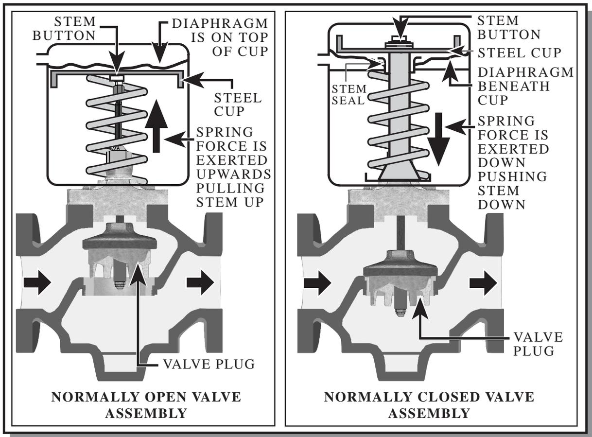
Normally open and normally closed are terms that refer to the position of an actuator and valve or actuator and damper assembly when the power is removed. Coils are prevented from freezing in an airhandler if the coil has full flow through it during the off cycle. Similarly a reheat coil on a variable air volume box does not require freeze prevention and the actuator should be closed if there is no airflow to prevent tripping plenum heat detectors.
