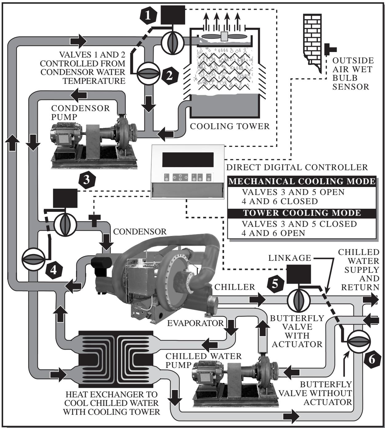
Heat exchangers can be used to cool a building using only the cooling tower. If the outside air humidity is sufficiently low the chiller can be turned off and just the tower fans and pumps energized. There is a substantial amount of rerouting of water flow required on typically larger pipe sizes so butterfly
