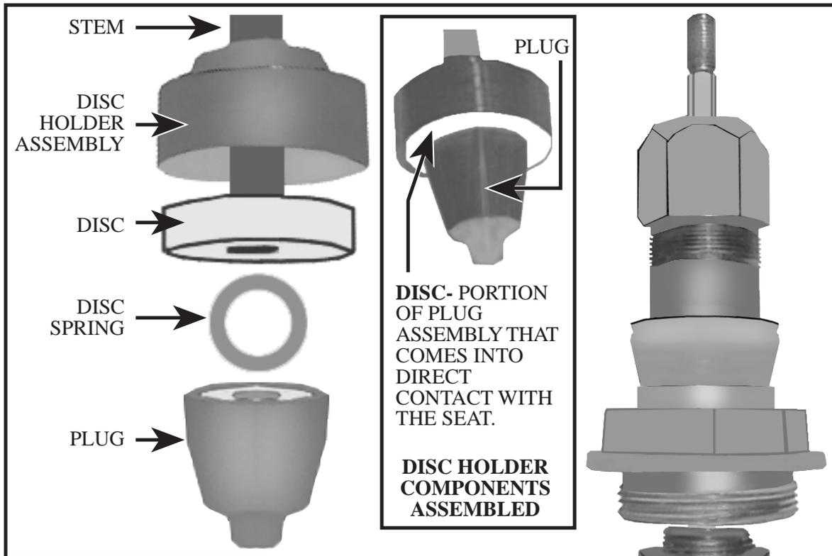
This is the configuration of a V5011 type of Honeywell valve. This is a 1 inch (25 mm) valve and the seat is removed with a deep thinwall 6 point socket wrench. On some of the stem-down-to-open valves the diameter of the seat exceeds that of the bonnet and a special Honeywell wrench is required that is inserted through the opening of the pipe. It is important to obtain the correct seat since there is more than one size for each valve. Installing the wrong one can alter the Cv of the valve.
