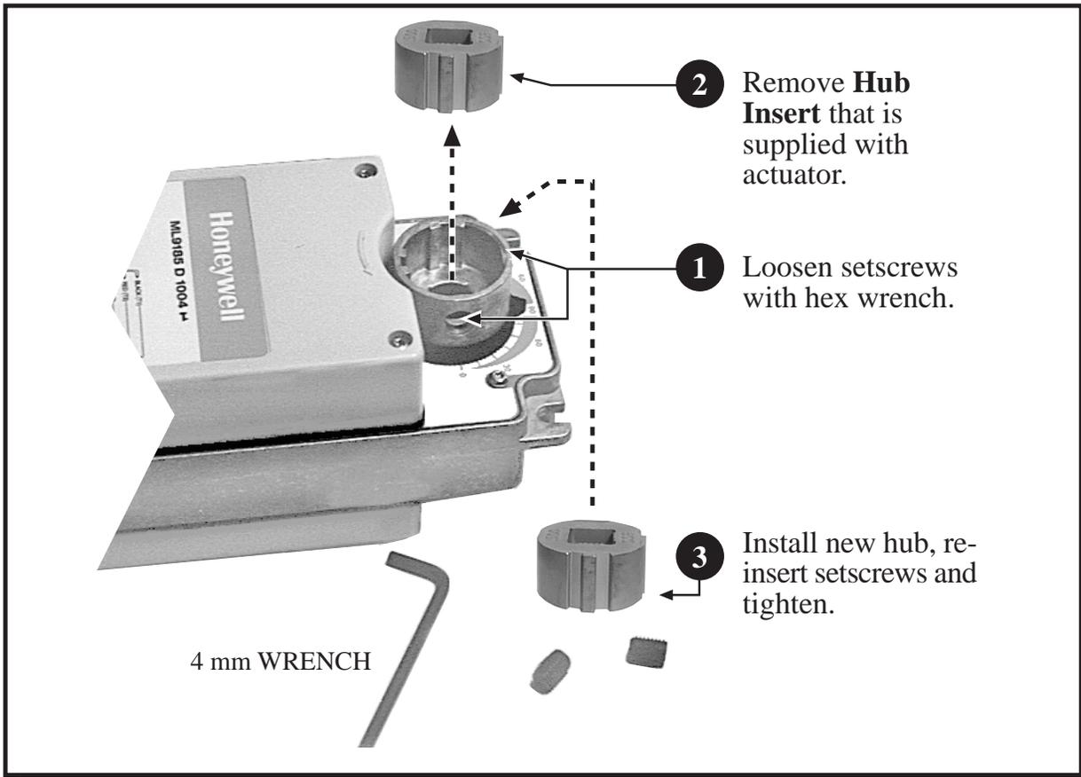
The hub insert is replaceable on the 50 lb-in (6 N-m) line of actuators. They are typically supplied with a 1/2 inch (13 mm) insert. There are three replacement hub inserts available. These are primarily for use with damper shafts and will probably not be used with ball valves since most ball valves linkages from Honeywell are either
