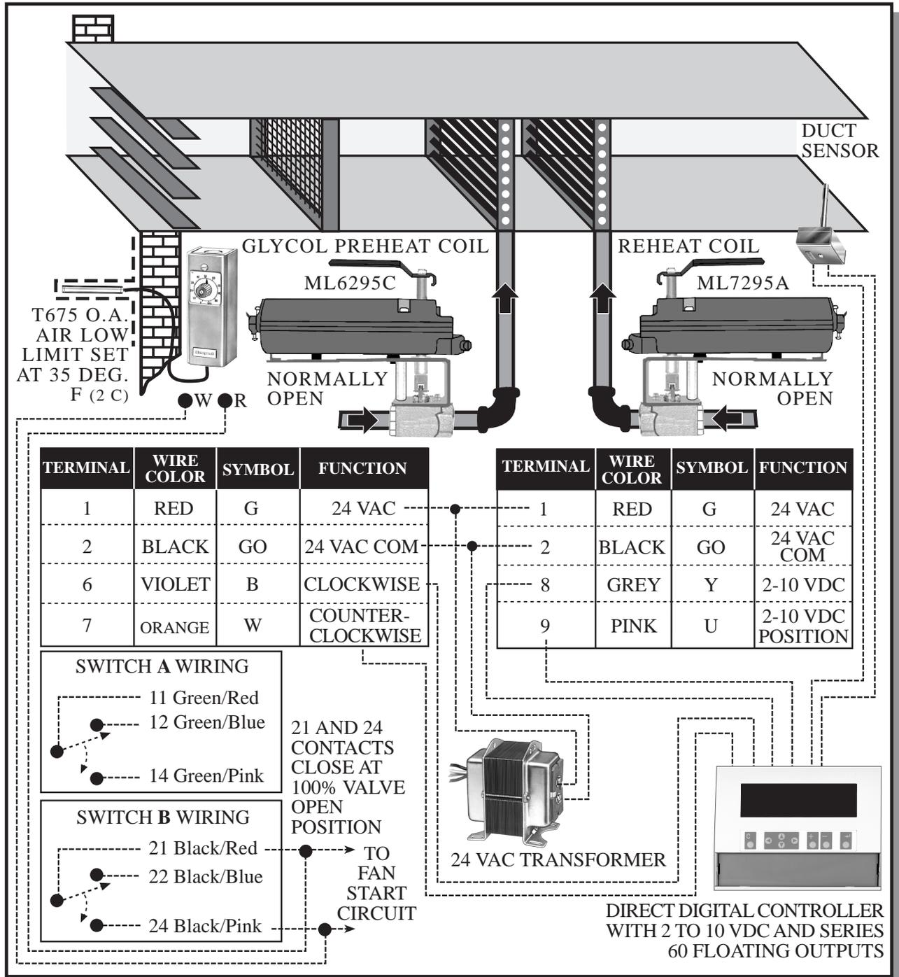
This is an airhandler with 100% outside air usage. There is a glycol preheat coil that must be opened fully whenever the outside air temperature is below 35 Deg. F. (2 C). This is accomplished with the direct digital controller. Additionally as a freeze avoidance measure the
