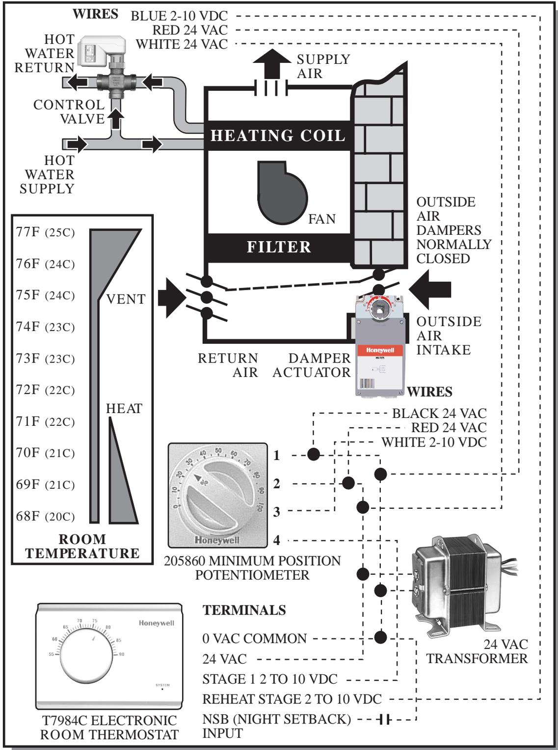
In warmer climates heating is required only for a short interval in the morning. A minimum position switch is used to ensure adequate ventilation at all times.
