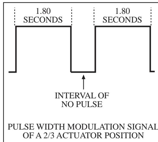
A pulse duration of 1.80 seconds would be 170 increments more than the minimum.
