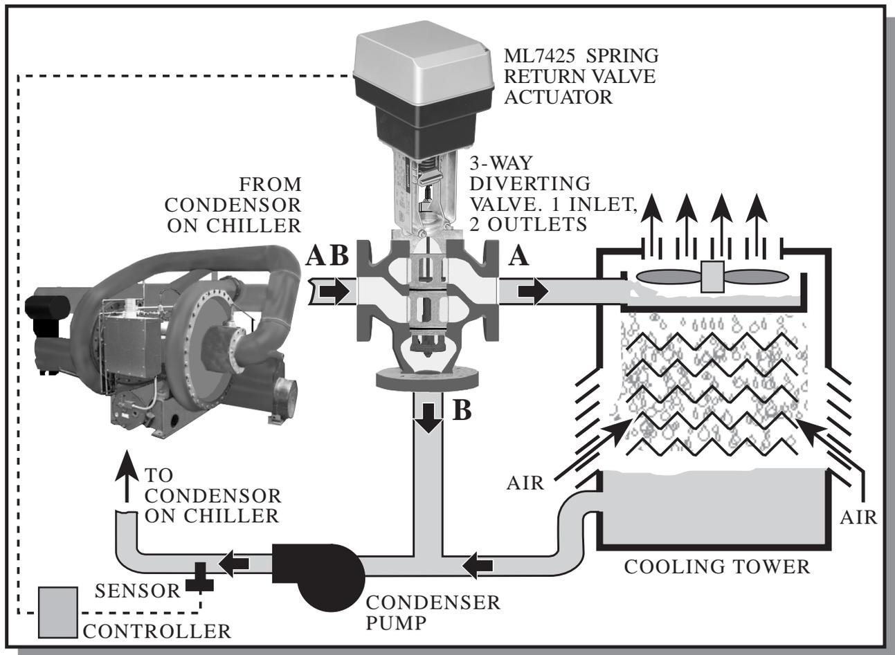
Chillers are used to generate chilled water to cool a building. While some of these are paired with air cooled condensers most of the larger units are connected to cooling towers. Cooling towers are used to dissipate the heat taken from inside of the building to the outdoors. A valve is generally required to control the temperature of the condensor water being returned to the chiller.
