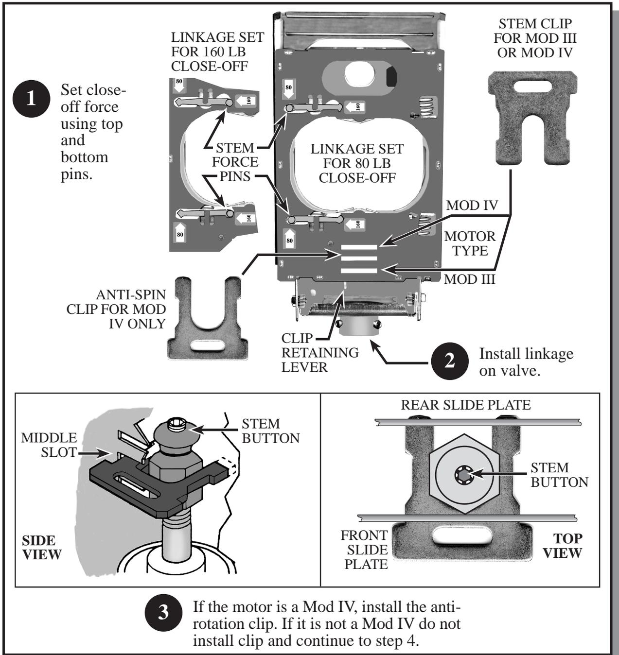
The Q5001 valve linkage is designed for installing Honeywell Mod III and Mod IV actuators on commercial globe valves. Stem force ratings of 80, 160 or 320 pounds are available depending upon the actuator. Stem lifts of 1/4 inch (.625 cm) to 1.5 inches (3.75
