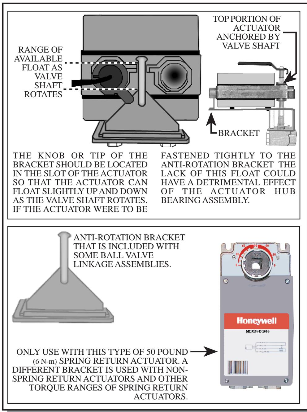
There are several ball valve linkages and each is designed to be used only with certain actuators. One or more anti-rotation brackets are included with the ball valve. These are designed to anchor the back of the actuator so it does not spin. It must
