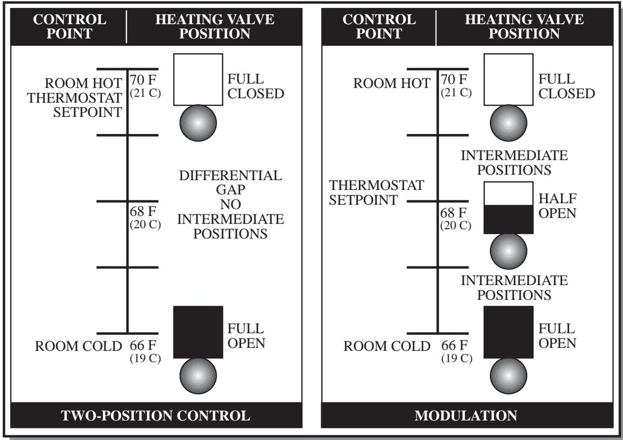
The most fundamental of control categories is 2-position or modulation. This indicates that the final control element is either full open or full closed with no intermediate positions. Most of these will use thermostats or controllers with single-pole-single-throw (SPST) or single-pole-double-throw (SPDT) switching. While this may appear to be a limited form of control it is adequate for many slow changing environments such as a room thermostat controlling a baseboard electric heater.
