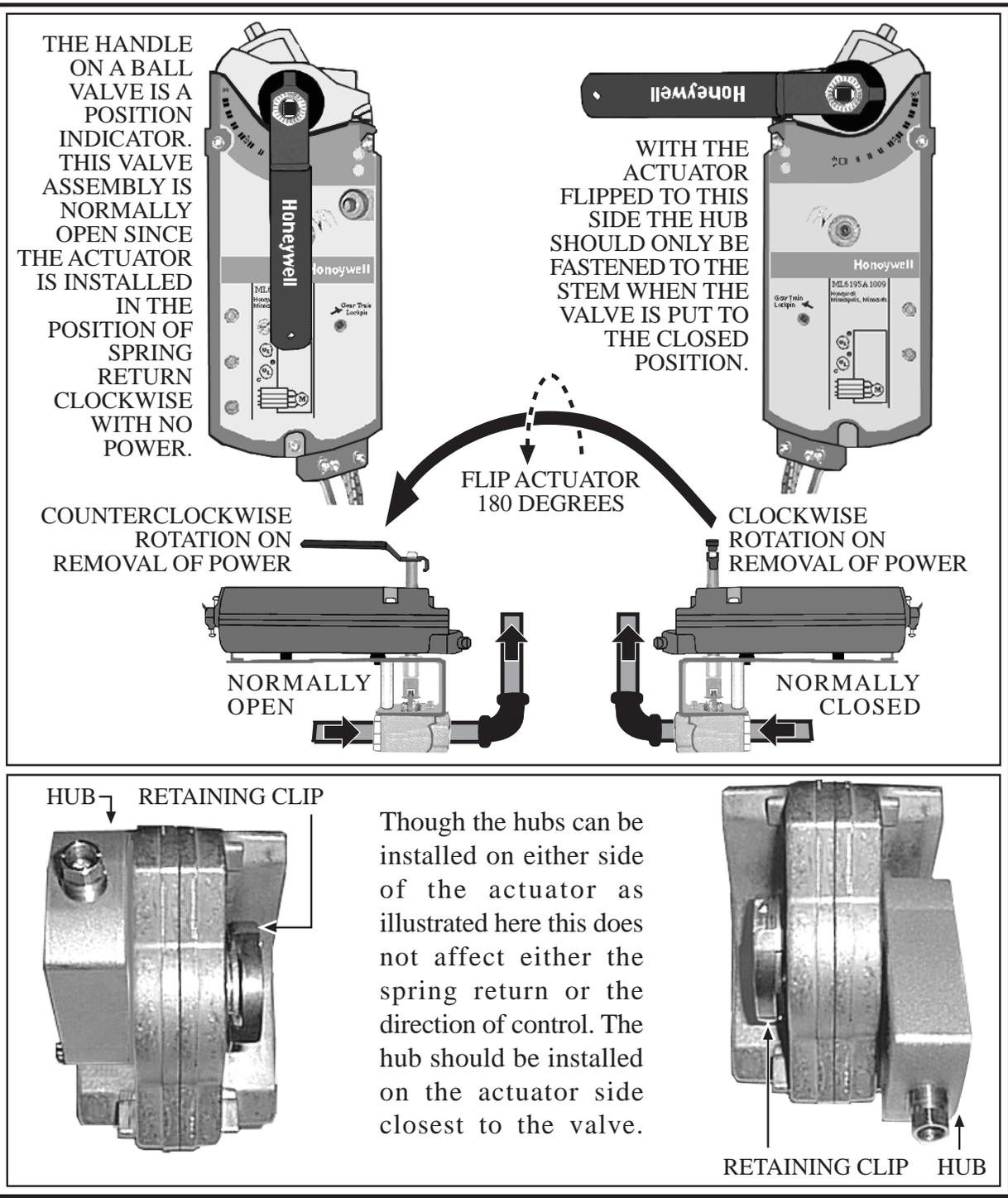
This actuator is reversed by flipping it 180 degrees. This reverses not only the direction of opening and closing but also the spring return. Since the actuator on the right spring returns in a different direction the hub must
