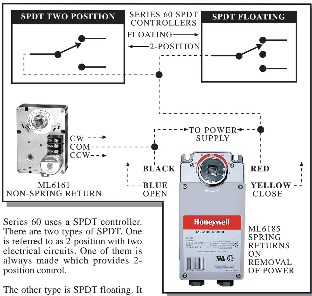
Series 60 uses a SPDT controller. There are two types of SPDT. One is referred to as 2-position with two electrical circuits. One of them is always made which provides 2-position control.
