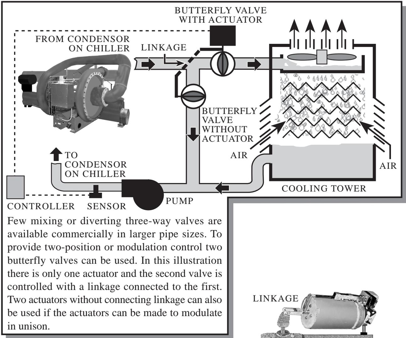
Few mixing or diverting three-way valves are available commercially in larger pipe sizes. To provide two-position or modulation control two butterfly valves can be used. In this illustration there is only one actuator and the second valve is controlled with a linkage connected to the first. Two actuators without connecting linkage can also be used if the actuators can be made to modulate in unison.
