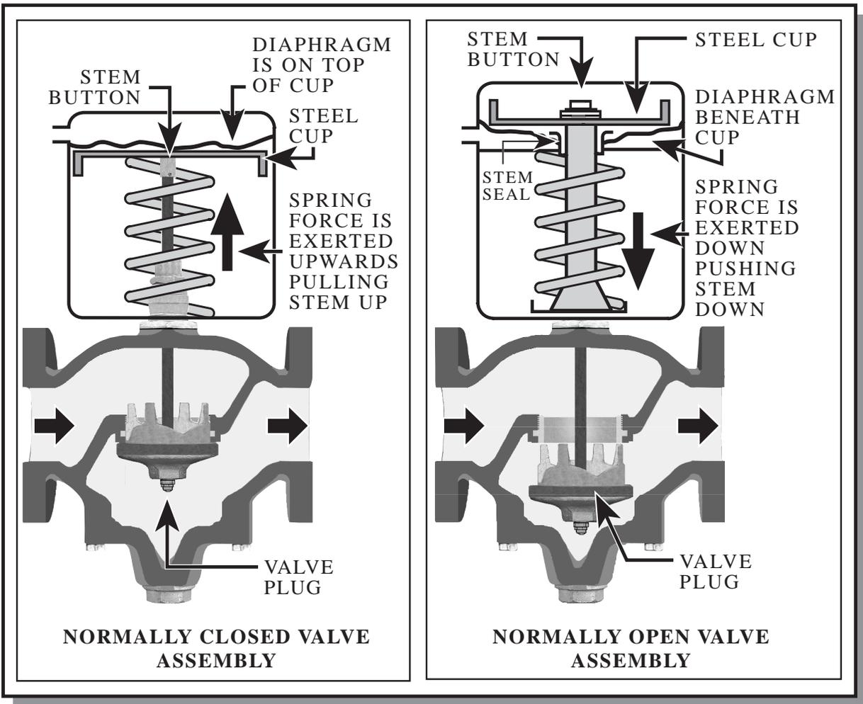
These are the same two actuators as on the previous page. The valve however is stem-down-to-open which reverses the normal position of the two assemblies.
