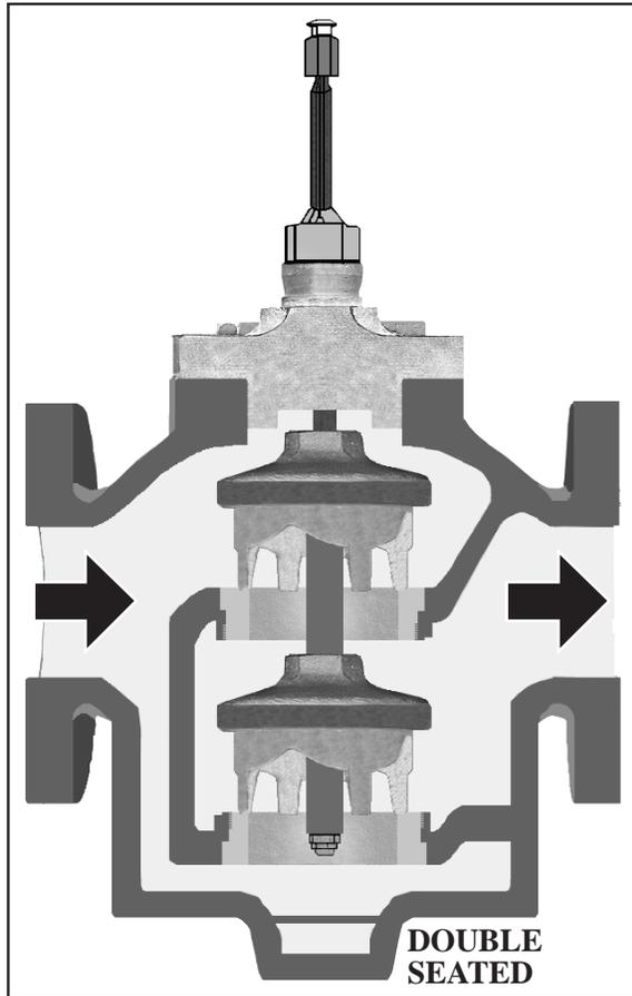
DISC IS JUST A FLAT PIECE. THERE IS FULL FLOW ALMOST IMMEDIATELY AFTER OPENING.
