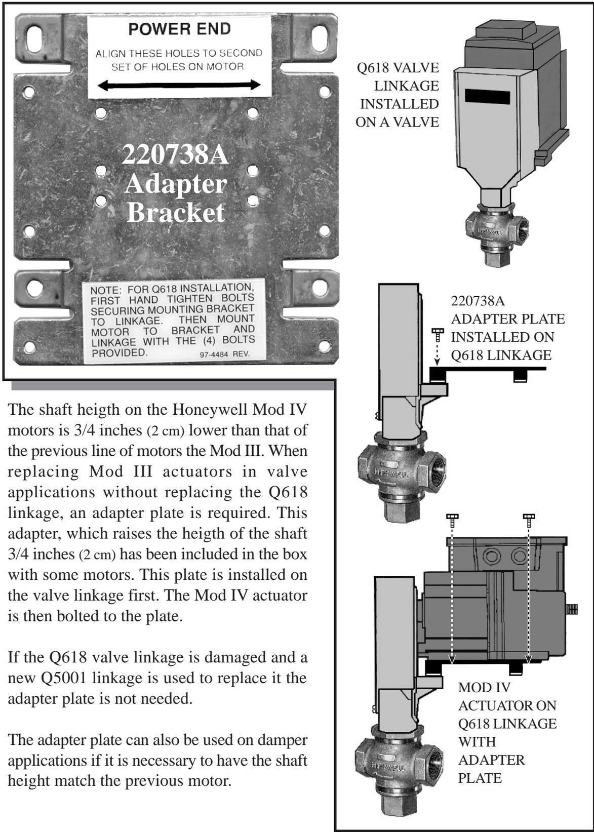
The shaft height on the Honeywell Mod IV motors is 3/4 inches (2 cm) lower than that of the previous line of motors the Mod III. When replacing Mod III actuators in valve applications without replacing the Q618 linkage, an adapter plate is required. This adapter, which raises the height of the shaft 3/4 inches (2 cm) has been included in the box with some motors. This plate is installed on the valve linkage first. The Mod IV actuator is then bolted to the plate.
