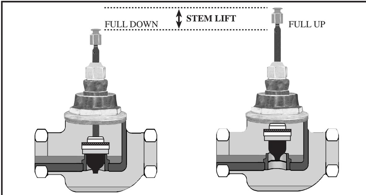
Valves are available as unitary or assembled units. The difference is that a unitary valve is designed to be used with a specific actuator. Unitary valves are typically smaller valves. An assembled unit consists of one of Honeywell's threaded or flanged valves and one of a wide selection of actuators. The actuator can be electric or pneumatic, spring return or non-spring return or one of any of the available close-off ratings.
