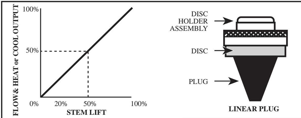
There are two primary types of plugs for globe valves. The one with straight sides is referred to as a linear plug and is used for modulating steam or chilled water. The other with the sloping sides is referred to as an equal percentage plug and is designed for modulation of hot water or two-position control of steam. It is equal percentage because each percentage of stem lift results in an equal percentage increase in heat output.
