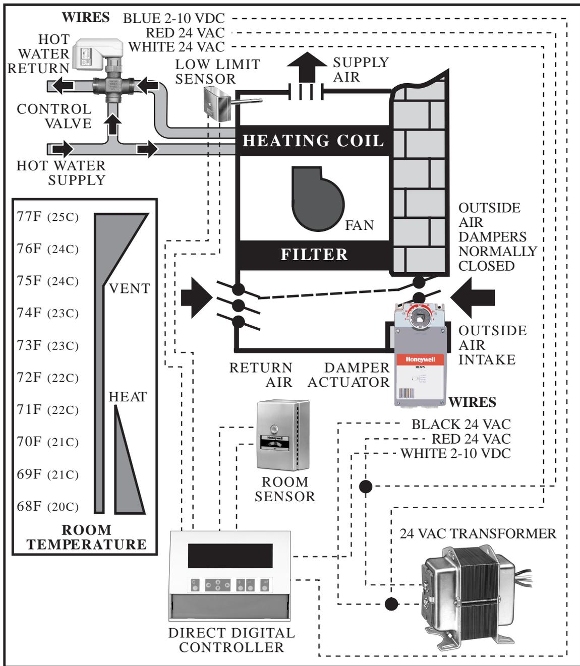
If the room becomes warm and the heating valve closed the supply air temperature can drop too low and cause cold drafts in the room. A supply air low limit prevents this by opening the heating valve if the supply temperature decreases below 55 or 60 Deg. F (13 or 16 C). Once the supply air temperature rises above the low limit
