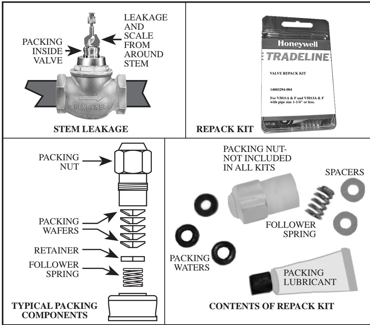
There are two primary types of valve servicing procedures: repack and rebuild. A rebuild is a more complete procedure and includes the entire repack procedure. Repacking is done more frequently and done equally as often on steam and hot water. Rebuild is done more frequently on steam valves.
