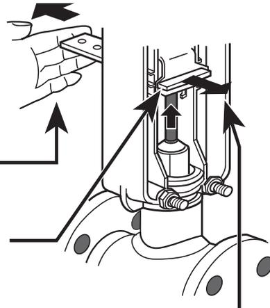
Release the stem button retaining clip to secure the stem button. Check to make certain the stem button is secured by the retaining clip.
