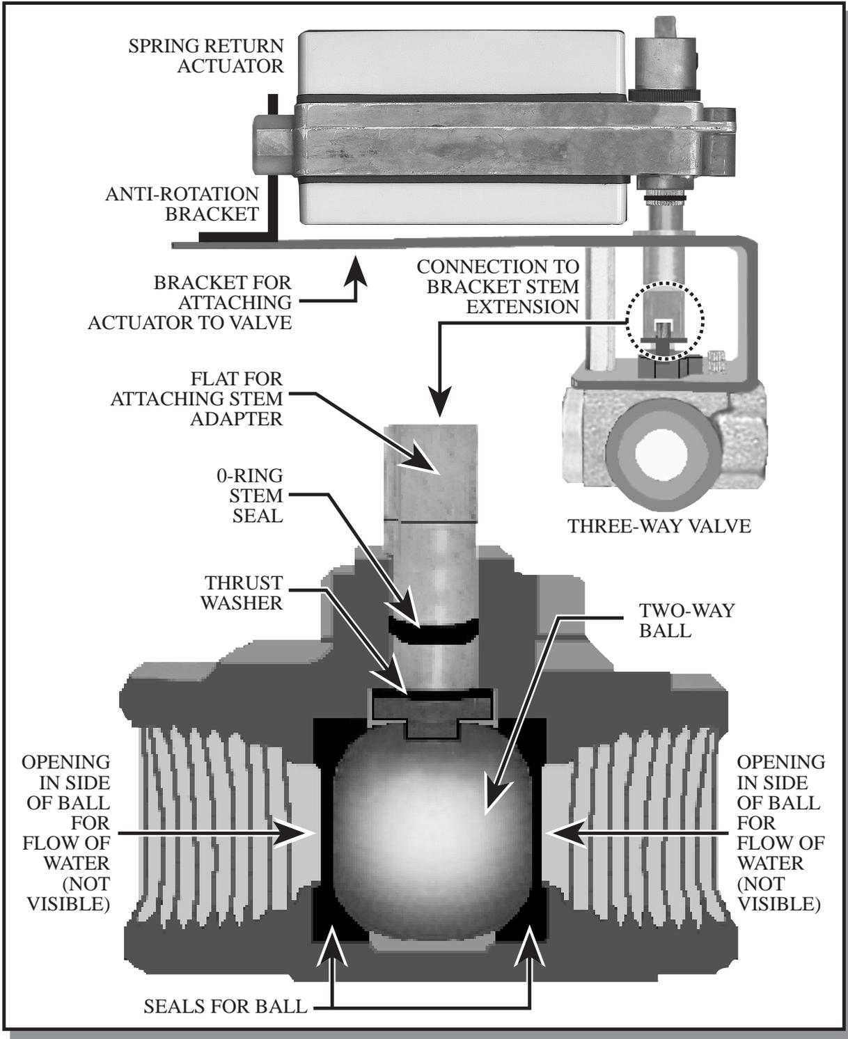
The bracket for ball valves is fastened to the top of the valve with bolts that are threaded into the body. The stem extension is fastened to the valve stem without any
