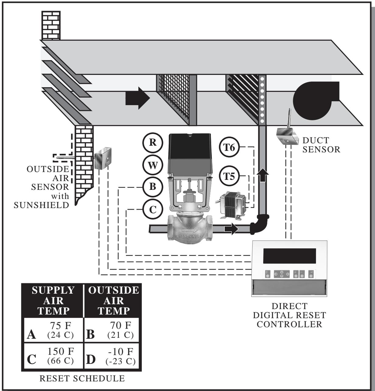
This is supply air reset of a heating coil on an airhandler using pulse width modulation. The actuator is a ML7984B used with a V5011 valve. Steam or hot water is supplied to the coil and the supply air temperature from the coil is varied with the outside air temperature to meet the needs of the
