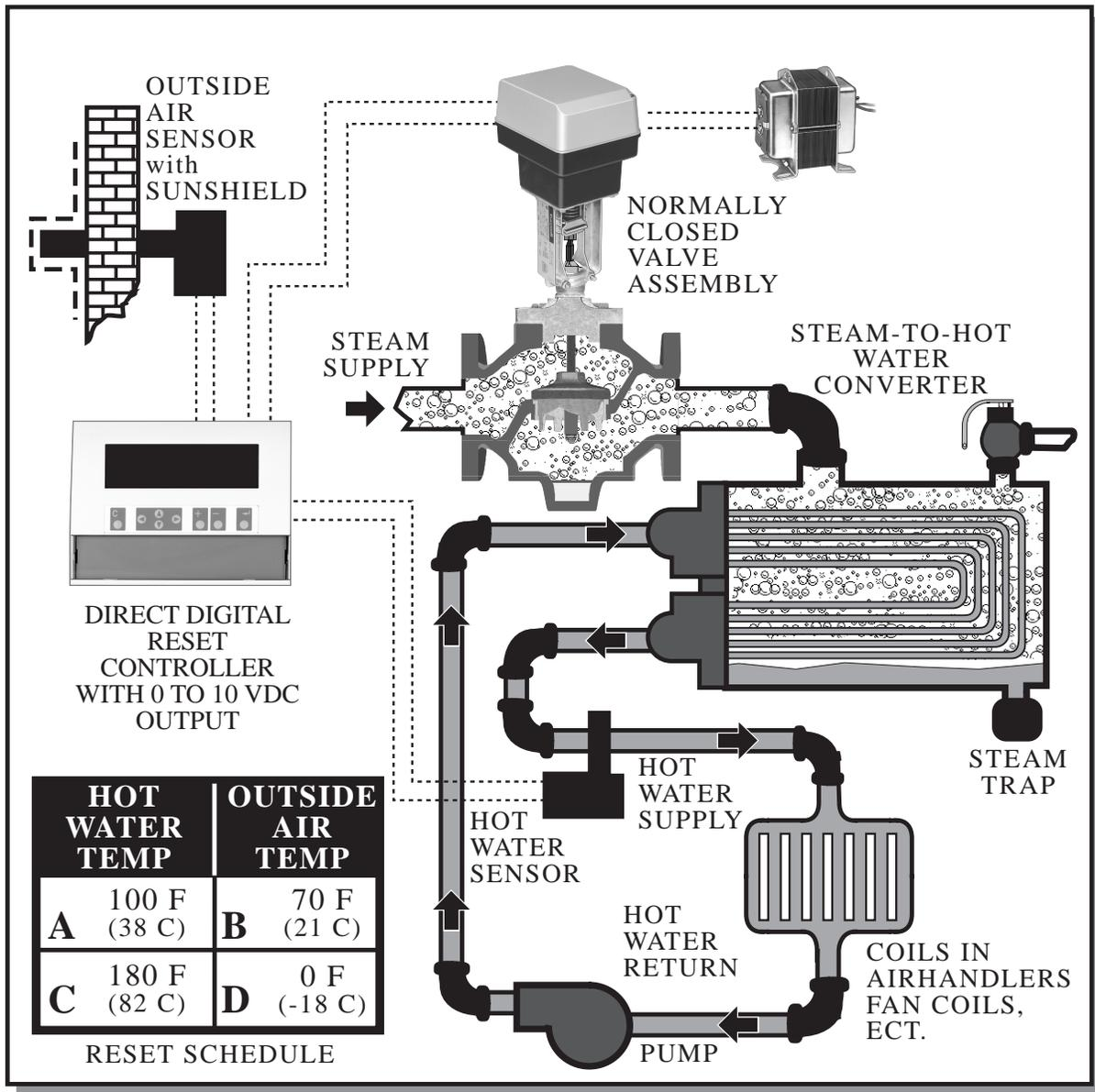
Most modern buildings are heated with hot water boilers. Facilities constructed prior to 1940 were probably heated with steam. Additions to these buildings are typically hot water heat due to its controllability, safety and maintenance benefits. The use of a steam-to-hot-water converter permits retaining the steam boiler while heating new areas of the building with hot water. Other facilities such as hospitals and industrial facilities often require the
