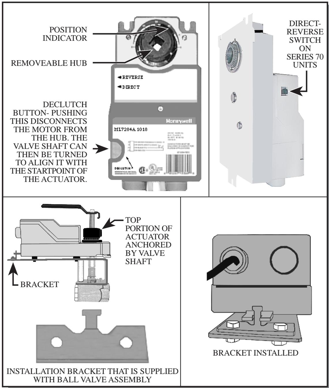
The non-spring return actuators are installed on the flat back side only. Direct-reverse adjustments are done on series 70 units with a switch on the side. The mounting hub is reversible but will protrude substantially when installed from the back. Hub inserts are available
