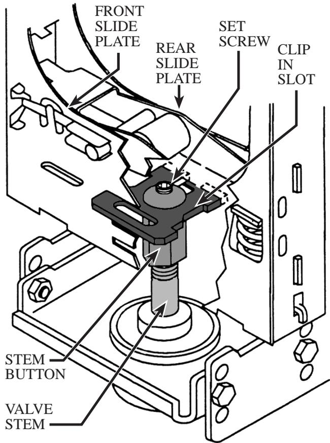
CLIP MUST ENGAGE SLOTS ON STEM BUTTON AND THE REAR SLIDE PLATE
