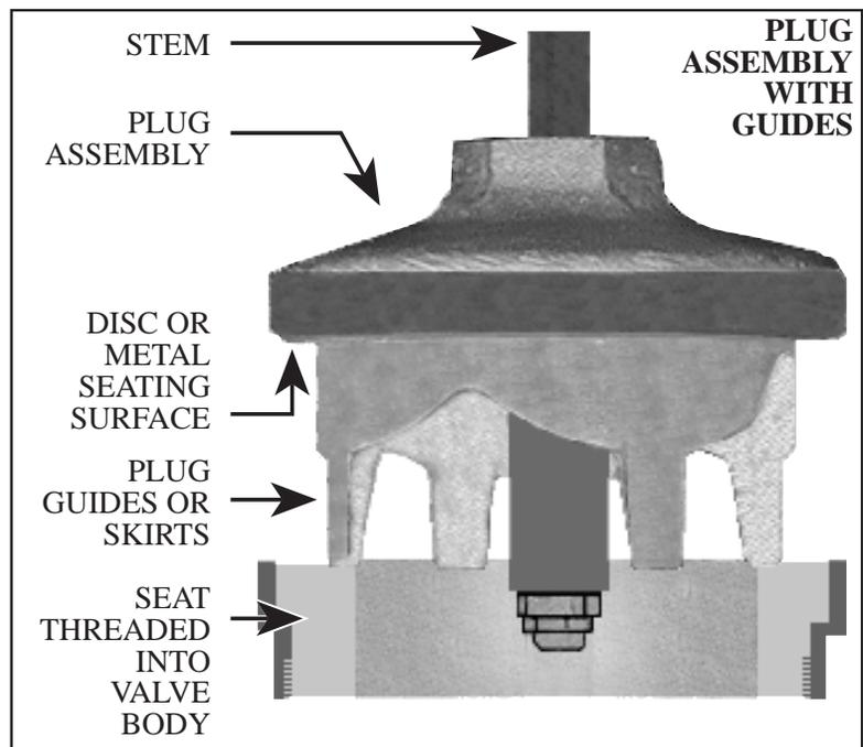
Both of the top two plugs on this page are constructed with discs that are used to make a tight seal with the seat to prevent leak through. Twenty years ago these seats were made of a fiber material referred to as composition, a rubber material for chilled water or metal for tight close-off with steam. Then the discs were changed to be made primarily of teflon or metal.
