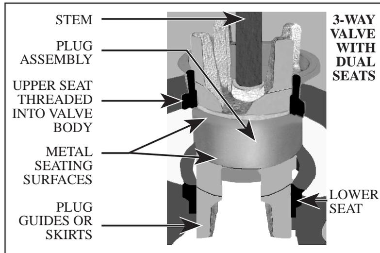
The three-way valve plug illustrated on the bottom is made without discs. Two seating surfaces are built into the plug assembly.
