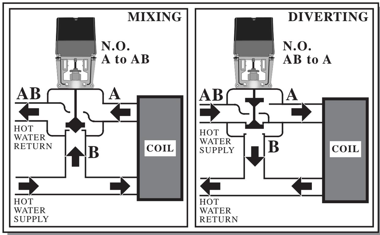
Three-way valves are primarily used for water applications and infrequently to switch compressed air. It is typically open to one port or the other. There are smaller three-way valves which sequence ports and can be closed or open to both ports simultaneously. Most of the larger valves though, are of the type illustrated here and would be labelled "Normally Open A to AB", or "Normally Open AB to B."
