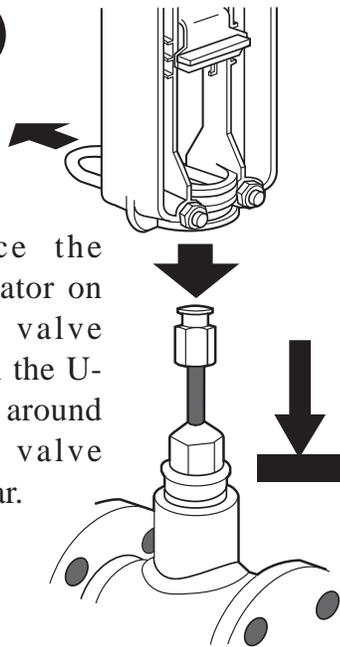
Place the actuator on the valve with the U-bolt around the valve collar.
