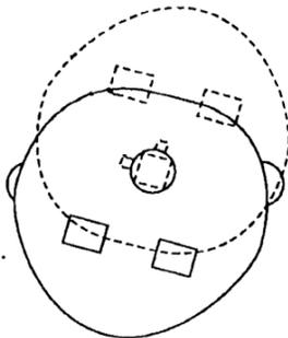
**5** Install cam on motor.
