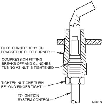
**Fig. 3. Always use new compression fitting.**
