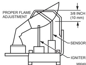
**Fig. 4. Sensor tip must be in pilot flame.**
