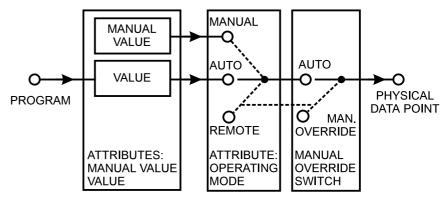
Fig. 20. Control flow for output functions
