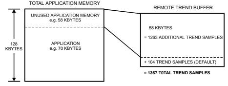
Fig. 25. Adjustable remote trend buffer example
