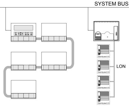
Fig. 4. Global data-points are available to all controllers on the system bus
