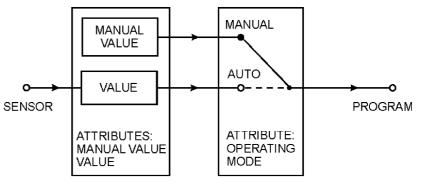
Fig. 17. Example of a sensor input
