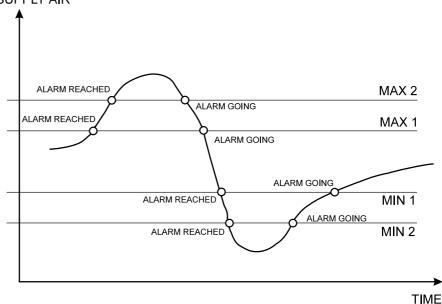
Fig. 10. Monitoring supply air temperature limits
