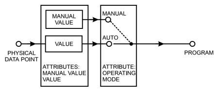
Fig. 19. Control flow for input functions
