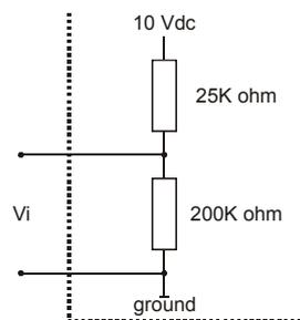
**Fig. 15. Analog inputs identified as DI point (O.S. 2.03.xx)**
