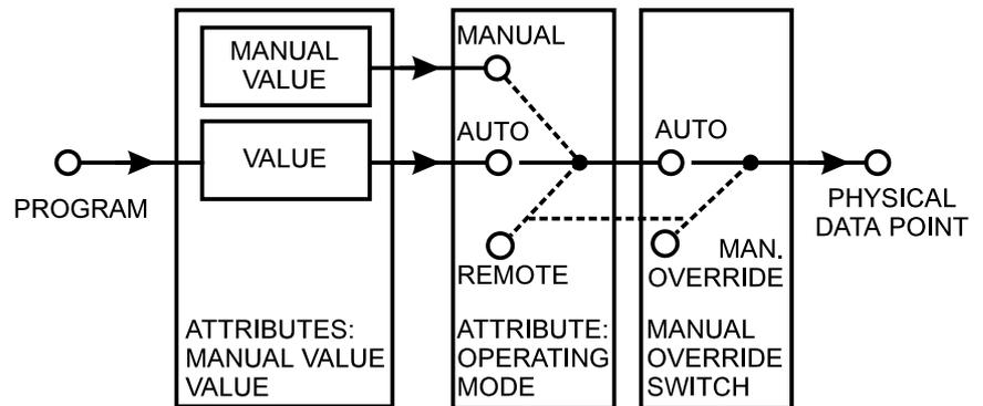
**Fig. 20. Control flow for output functions**
