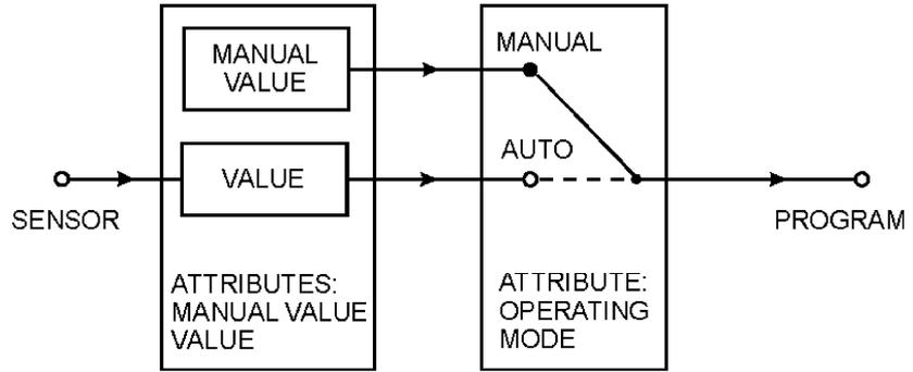
Fig. 17. Example of a sensor input
