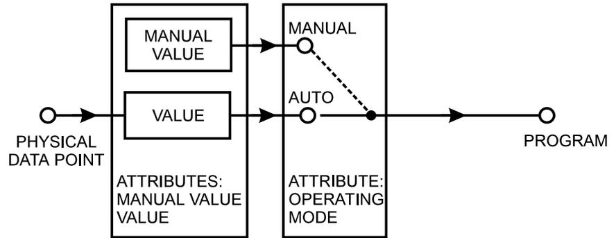
**Fig. 19. Control flow for input functions**
