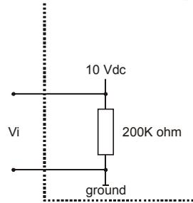
**Fig. 14. Analog input / high-impedance sensors**
