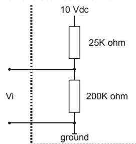
**Fig. 1. Analog input / low-impedance sensors**
