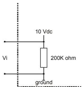
Fig. 16. Analog inputs identified as DI point (O.S. 2.04.00 or higher)
