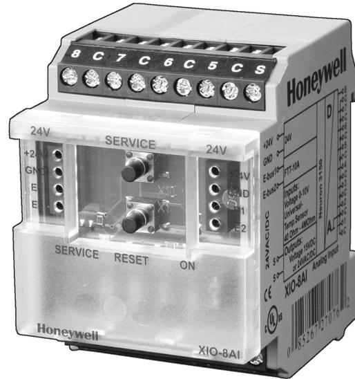
The XIO-8AI Analog Input Module has 8 inputs, which can be wired to passive resistance sensors or active sensors (voltage inputs) as needed. For active sensors, the permissible input D.C. voltage is 0 to 10 V. Resistance sensors can work in a range of 40 Ohm to 4 Megohm. The setting of the ranges and input of the sensor characteristic curves with 10 support points for linearization is performed with an LNS® plug-in.
