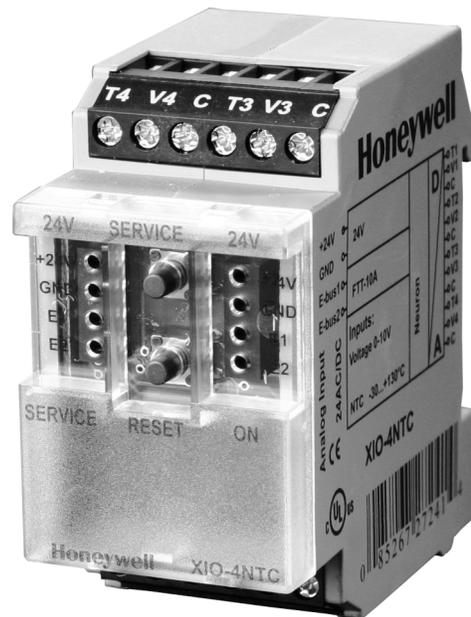
The XIO-4NTC LON Analog Input Module is a LON module with 8 analog inputs, 4 temperature and 4 voltage, suitable to collect temperature data with NTC 20K sensors and voltage values. In a LON installation, all 8 inputs can be scanned simultaneously by standard network variables, SNVT.
