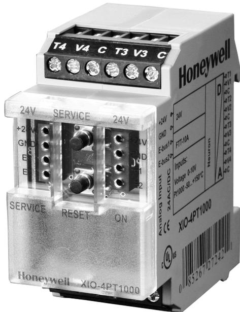
The XIO-4PT1000 LON Analog Input Module is a LON module with 8 analog inputs, 4 temperature and 4 voltage, suitable to collect temperatures with PT 1000 sensors and voltages. In a LON installation, all 8 inputs can be scanned simultaneously by standard network variables, SNVT.
