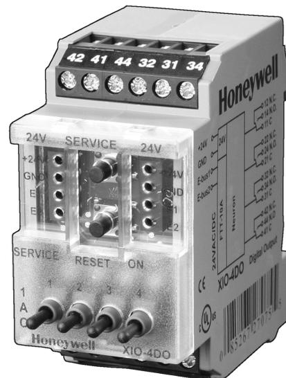
The XIO-4DO Digital Output Module is used to switch electrical units, such as fans, pumps, etc. Four independent relays with one potential-free change-over contact are available for this purpose.
