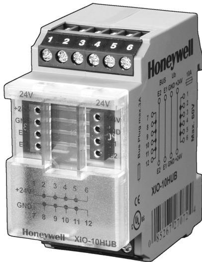
The XIO-10HUB Terminal Module provides additional support terminals, e.g., for the power supply of external drives. The terminals are not connected to the internal 24 V and ground wires; thus, they can be used individually. Six (6) terminals each are bridged among each other.
