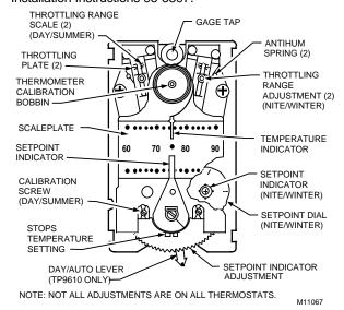
Fig. 3. TP9600-TP9630 thermostat with cover removed.
