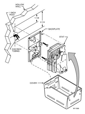
Fig. 4. Installing TP9600 - TP9630 without wall box.
