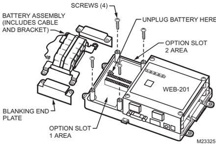
**Fig. 2. Removal of screws and battery assembly.**
