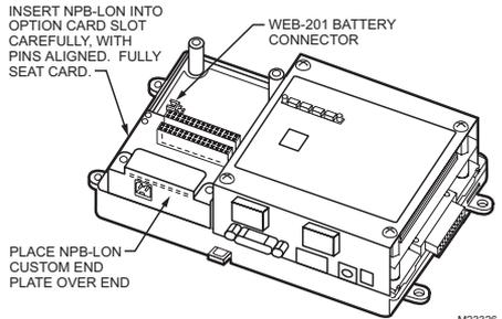
**Fig. 3. Top view, NPB-LON end plate insertion.**
