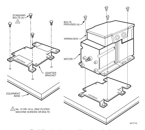
Fig. 3. Mounting the motor with an adapter bracket.
