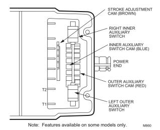
Fig. 5. Terminals and adjustments.
