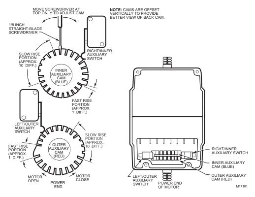
Fig. 13. Auxiliary switch adjustments.
