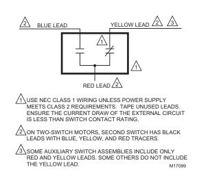
Fig. 12. Auxiliary switch schematic.
