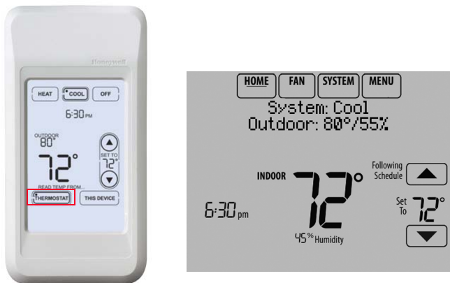
Fig. 302. Reading temperature at the thermostat.
