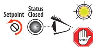
3. Turn the screw an additional 1/4 turn counter-clockwise for operational margin.
