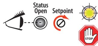
3. Turn the setpoint screw an additional 1/4 turn clockwise for operational margin.
